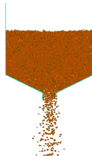
Fig. 6. Hopper discharge of a well-mixed initial fill.
