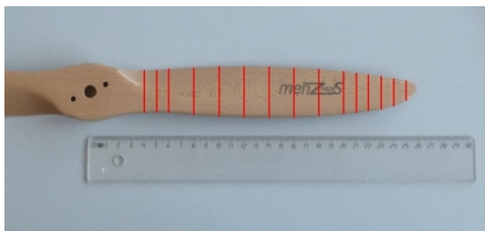
(e) Propeller cutting to get precise geometrical data
