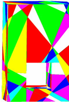
Figure 2.3.1: 3D model of a rectangle excavation and its vicinal blocky rock mass generated on RESOBLOK
