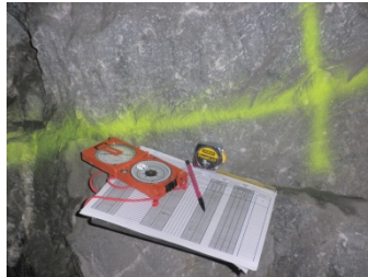
Figure 2.1.2: Trace of a scan-line on an underground rock face
