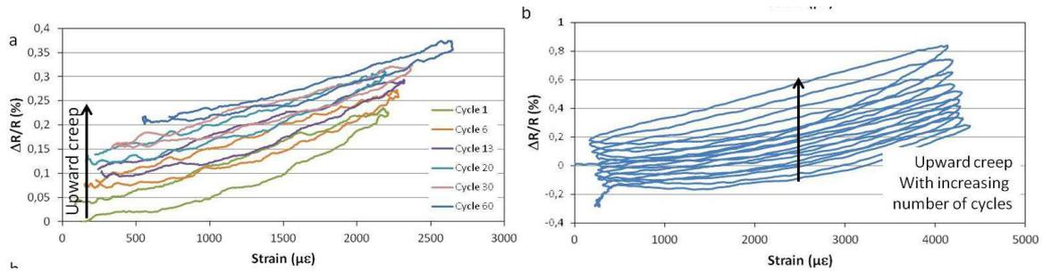
Figure 6: Resistance-strain curves of a CNT strain sensor during high strain load cycles: a) 4N, 2500 $\mu\epsilon$ , 10s period ; b) 8N, 4000 $\mu\epsilon$ , 5min period
