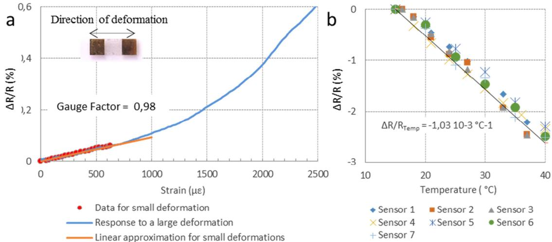
Figure 5 a) Resistance variation with respect to strain. The linear regime reaches up to 700  $\mu\epsilon$  for this device. The gauge factor of the device presented here is 0,98. Overall, the response up to large strains is roughly quadratic. b) Linear dependence of resistance on temperature. The temperature sensitivity is equal to  $-1.0 \times 10^{-3} \text{ K}^{-1}$ .
