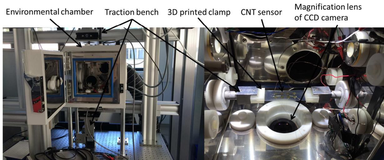
Figure 24: Platine dedicated environmental chamber with integrated traction bench and high-resolution optical imaging.
