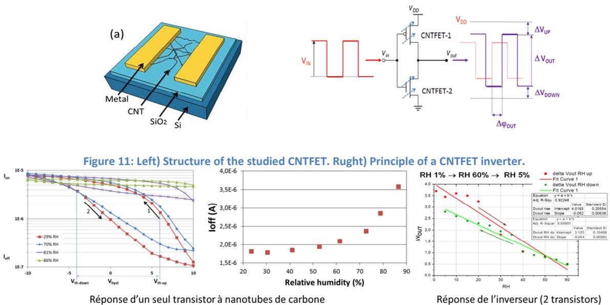
Figure 11: Left) Structure of the studied CNTFET. Right) Principle of a CNTFET inverter.
