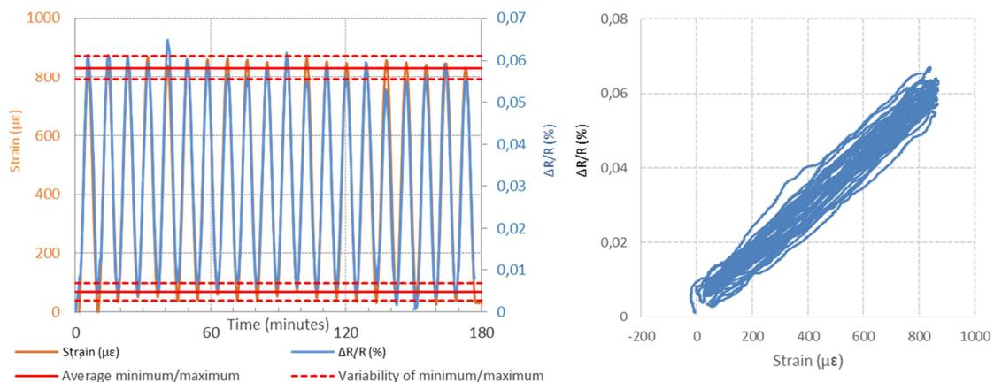
Figure 25 a) Response of a CNT strain sensor to 20 cycles of strains between 0 and 800  $\mu\epsilon$ . No evident hysteresis or baseline drift is observed. b) Corresponding resistance-strain plot. The extent of the bundle of resistance-strain curve is due to a slight variability (4.7%) in min and max resistance value. It is attributed to temperature variations in the range of approx.  $\pm 0.3$   $^{\circ}\text{C}$ .
