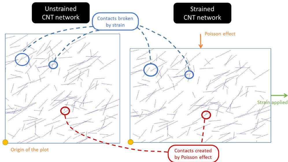
**Figure 29: Schematic of the CNT network under elongation. On the left, the simulated network unstretched. On the right, the simulated network elongated along the horizontal direction and consequently shrunk in the vertical direction due to the Poisson's effect.**
