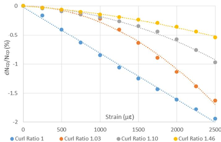
Figure 36: Simulation results showing the relationship between variation of number of contacts ( $dN_{pixel}/N_{pixel}$ ) and applied strain for different curl ratios. Curl ratio=(CNT length)/(effective CNT length) [Li 2007]
