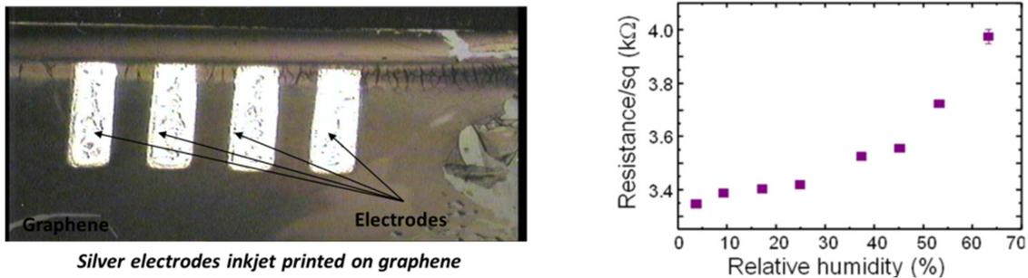
Figure 10: Humidity sensing with interfacial graphene on glass
