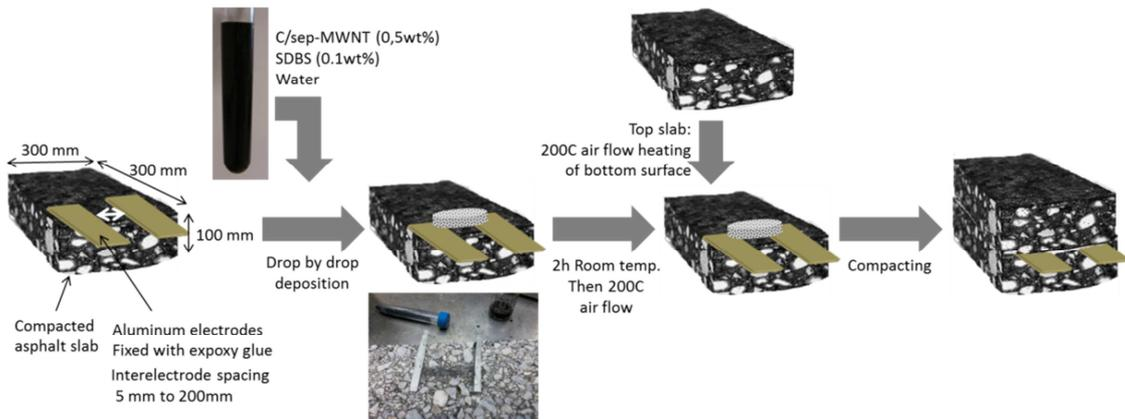
Figure 17: The asphalt sandwich: fabrication process. A layer of C/Sep-MWCNTs particles is deposited directly on a precompact asphalt slab and a pair of electrodes.
