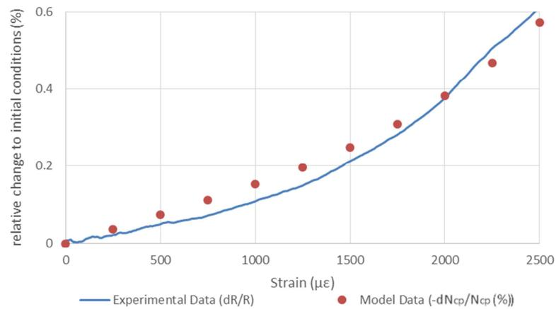
Figure 35: Comparison between model and experimental data for large deformation (2500  $\mu\epsilon$ ).
