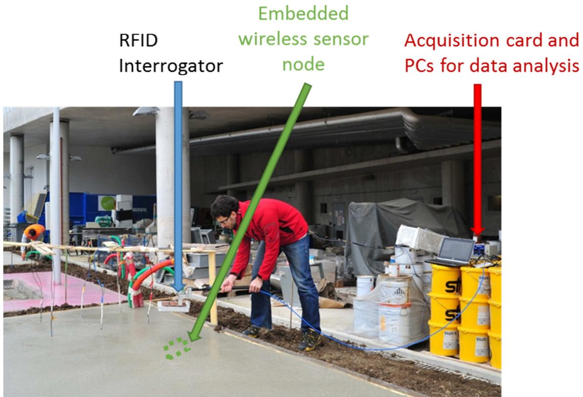
Figure 22 : Fulvio Michelis interrogating an embedded RFID tag right after casting of the concrete slab.
