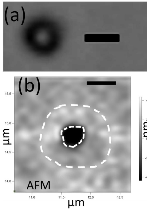
Figure 38 - Morphology of laser-annealed vnC-G. (a) Optical image (scale bar  $1\ \mu\text{m}$ ) of a laser-annealed region with energy density  $5.9 \cdot 10^6\ \text{J} \cdot \text{mm}^{-2}$  (b) AFM 2D height image showing a crater (black surrounded by a white dashed line) and a surrounding bulge (marked with a white dashed line) of a laser-annealed region with energy density  $1.7 \cdot 10^7\ \text{J} \cdot \text{mm}^{-2}$
