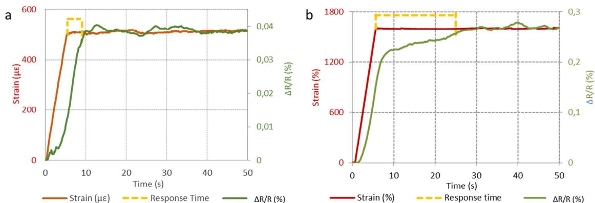
Figure 6 Measurement of device response time: a) 3.6 s under small strains (500  $\mu\epsilon$ ). b) 19 s under large strains (1500  $\mu\epsilon$ ).
