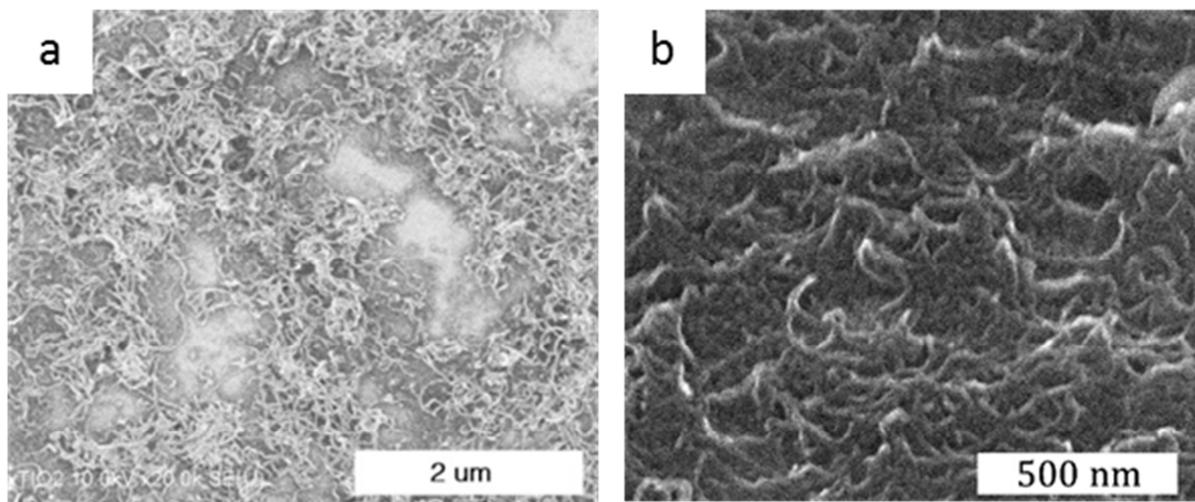
**Figure 30: a) SEM image of 1-layer deposition. Micrometric holes are observed in the layer; they are attributed to loss of matter during rinsing. b) SEM image of 20-layer deposition. A uniform coverage can be observed.**
