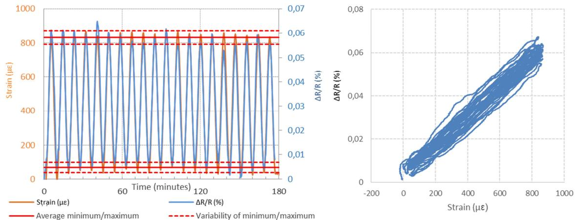
Figure 7 a) Response of a device to 20 cycles of strains between 0 and 800  $\mu\epsilon$ . No evident hysteresis or baseline drift is observed. b) Corresponding resistance-strain plot. The extent of the bundle of resistance-strain curve is due to a slight variability (4.7%) in min and max resistance value. It is attributed to temperature variations in the range of approx.  $\pm 0.3^\circ\text{C}$ .
