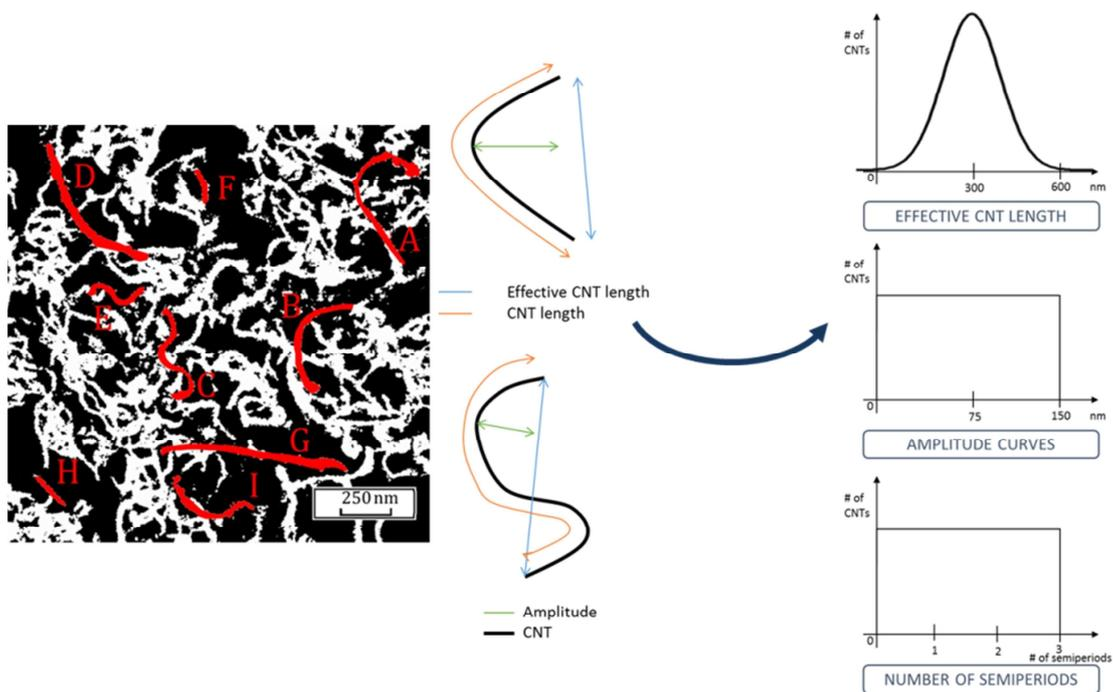
Figure 33 : Left) Naked-eye extraction of CNT and estimation waviness parameters (effective length, amplitude of curves, number of semiperiods) on a SEM image of the CNT network Middle) Definition of CNT waviness parameters Right) Distribution of CNT parameters used in the model
