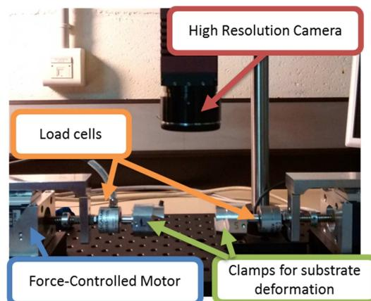
Figure 2 Extensometric bench used for electromechanical characterization.
