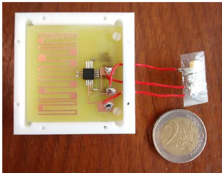
**Figure 21: CNT strain sensor assembled with its conditioning electronics and its RFID tag for concrete monitoring. All the electronics beside the sensor itself is enclosed into a protective Teflon box with silicon sealing.**
