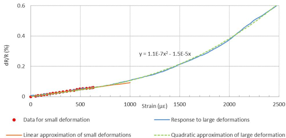
**Figure 15: Piezoresistive behavior of a CNT network-based strain sensor. The linear regime reaches up to about 700  $\mu\epsilon$  here. The average gauge factor is  $0.9 \pm 15\%$  over 8 devices.**
