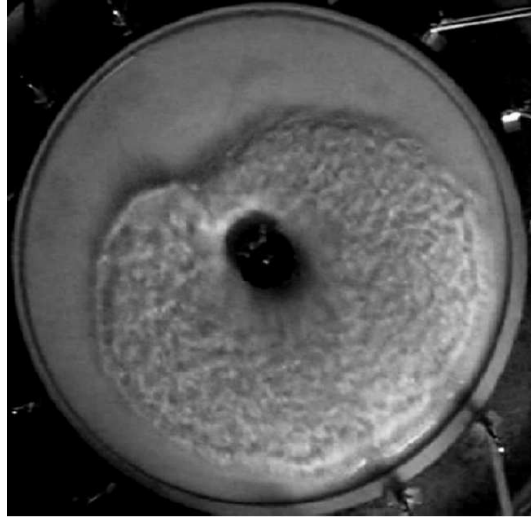
Fig. 1.9 – The shape of the rotating hydraulic jump observed in the SWASI experiment. The rotating singular (angular) point occurs as a result of non-linear behavior of the free surfaces.
