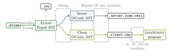
Figure 6.2: The ELIOM pipeline
