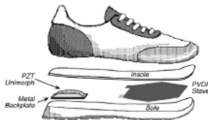
Fig. 1.6. Schematic and results of energy harvesting shoe.[ KYM 1998 ]
