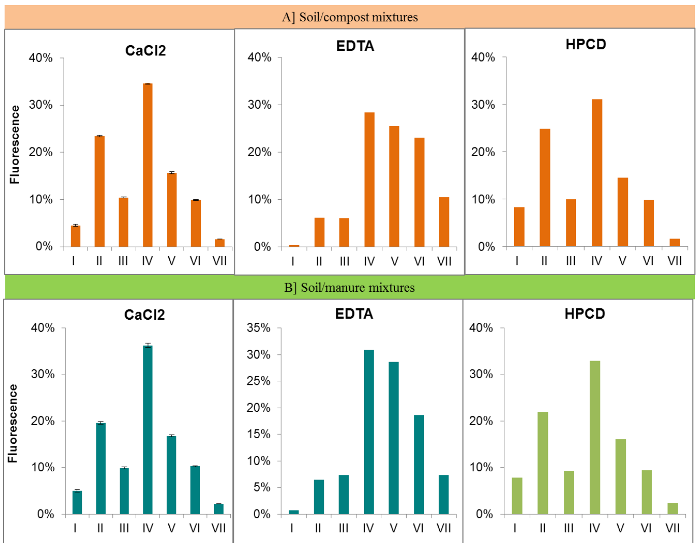
Figure IV.S1. Fluorescence (%) measured in the different zones in CaCl 2 , EDTA and HPCD extracts of A] soil/compost mixtures and B] soil/manure mixtures at day 0.
