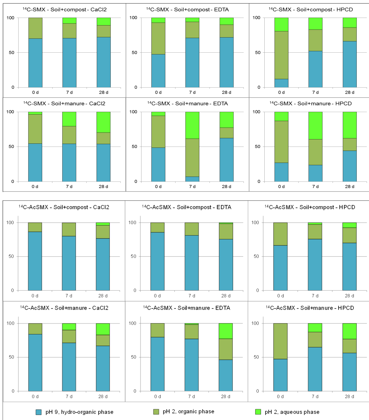
Figure III.S2. Partitioning of the ^{14}\text{C} -activity (% solvent-extractable; average, n = 3 ) between hydro-organic phase (pH 9), organic phase (pH 2) and aqueous phase (pH 2), for ^{14}\text{C} -AcSMX or ^{14}\text{C} -SMX in soil/compost and soil/manure mixtures. CaCl 2 , EDTA and HPCD referred to the soft extractant used before the solvent-based extraction.
