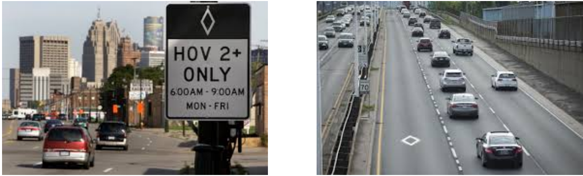
Fig. 2.2: Examples of high-occupancy vehicle (HOV) lanes
