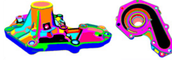
Fig. 7: Segmentation results of the pump cover
