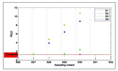
Figure 4.14 – Example of different faults exclusion using *PKLD*.
