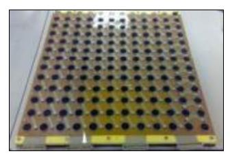
Figure 2.15 – The structure of the FSR floor presented by Gouwanda and Senanayake.
