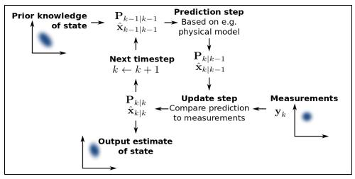
Figure 4.1 - Kalman filter schema: prediction and correction phase.
