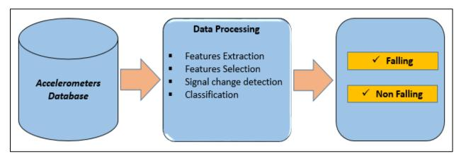
Figure 3.35 - Falling detection using accelerometer.
