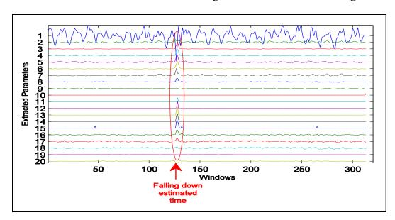
Figure 3.21 - Some Extracted Parameters (1: TR, 2: DFA, 3-7: Wavelet Packet decomposition parameters, 8: MPF, 9-18 Decil, 19: SE, and 20: LE).
