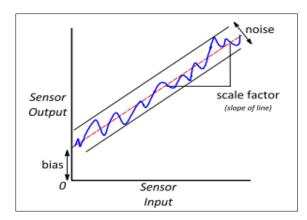
Figure 4.3 - Some of IMUs erroneous measurements.
