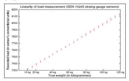
Figure 3.3 – The load measure linearity for a tile. The intervals that can be seen instead of expected dots are due to measurement noise.
