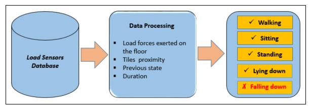
Figure 3.14 - ADLs recognition using simple pressure sensors.
