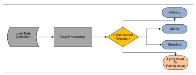
Figure 3.36 – ADLs recognition using load dada.
