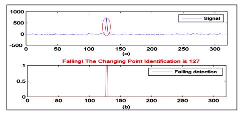
Figure 3.31 – Parameter changing detection when a fall occurs.
