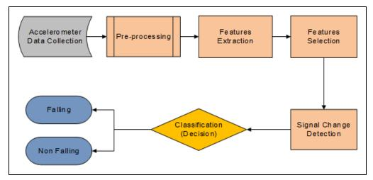
Figure 3.17 – The accelerometer data processing steps.
