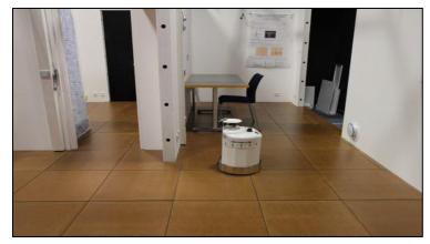
Figure 2.26 – PeKeeII robot communicating with an interactive sensing floor.
