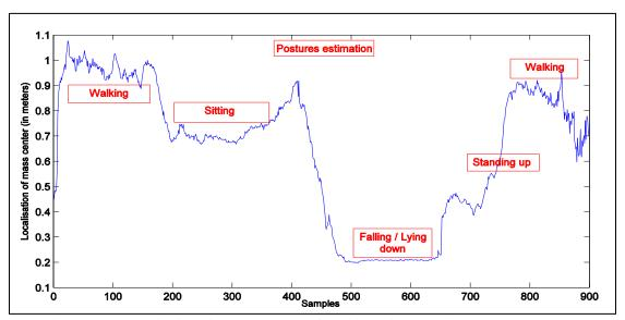
Figure 3.13 - Localization of the mass center of a subject with the estimated postures results.
