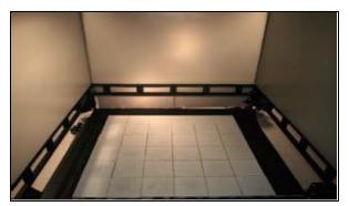
(a) The floor pressure-sensing interface.
