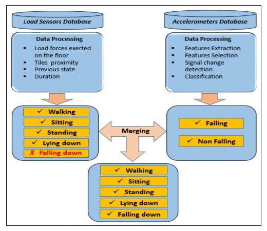
Figure 3.39 – ADLs recognition and fall detection.
