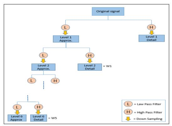
Figure 3.19 - Wavelet packet decomposition.
