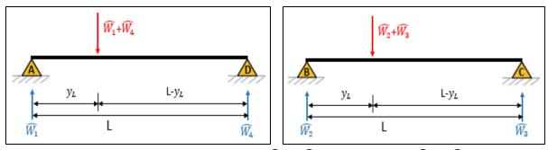
Figure 4.5 - The weight (W) is divided into two parts:  $(\widehat{W}_1 + \widehat{W_4})$  on [AD] (left) and  $(\widehat{W}_2 + \widehat{W_3})$  on [BC] (right).
