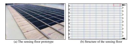
Figure 2.11 – The sensing floor which employs BOCDA technology.
