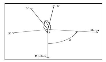
Figure 2.5 - Rotation of gravity relative to fixed coordinate.
