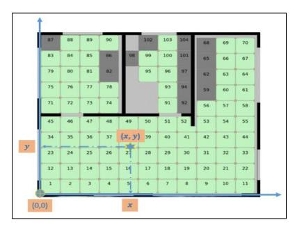
Figure 4.6 - The position coordinates of a person in the platform plan.
