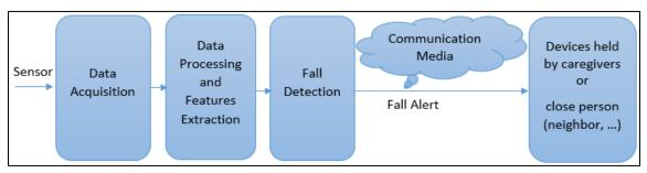
Figure 2.2 - General framework of a fall detection system.
