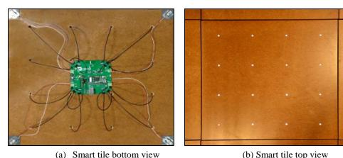
Figure 2.24 – The smart tiles. The bottom view (a) shows the pressure sensors located in the corners, as well as the accelerometer and the CPU visible in the center. The black cables feed 16 light emitting diodes (LEDs) that are used for providing visual feedback and shown in top view (b).
