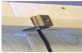
(b) An enlarged view of the load cell supporting
