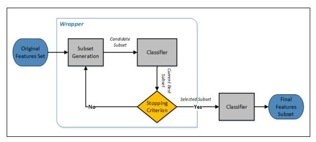
Figure 3.25 - Procedure of the wrapper model.
