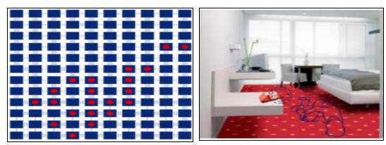
Figure 2.10 - Sensor signals (left) derived from a person that lies on the smart carpet prototype like depicted in the right picture.
