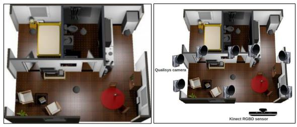
Figure 2.23 - The Inria Nancy smart apartment (left), the location of the 8 cameras of the Qualisys system and the Kinect camera (right).
