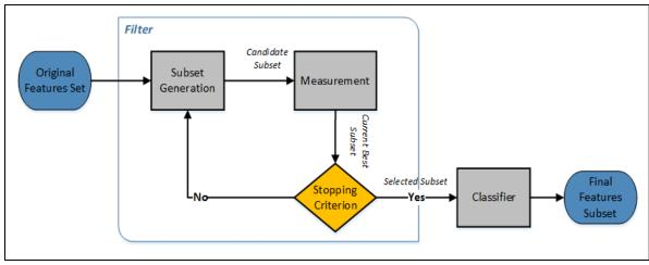
Figure 3.24 - Procedure of the filter model.
