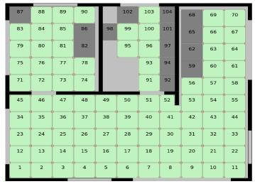
Figure 2.25 - Cartography of the tiles composing the sensing floor, with their identifiers.
