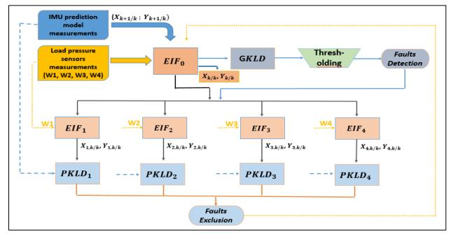
Figure 4.7 – The detection and exclusion procedure of defect.
