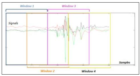
Figure 3.18 - Windowing process.
