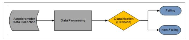
Figure 3.37 – Fall detection using accelerometer dada.
