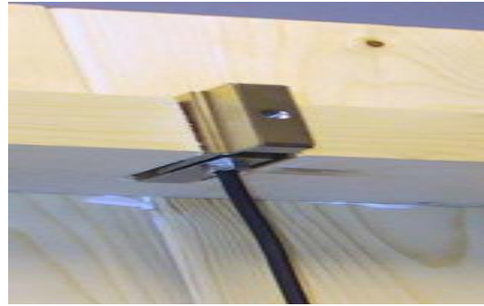
(b) An enlarged view of the load cell supporting the floor
