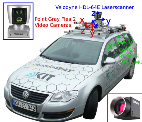
FIGURE 1.2 – Example of a 2D-and-3D camera system [1] rigidly mounted on a mobile platform. Such system contains a Flir color camera (red bounding box) and a Velodyne 3D laser scanner (blue bounding box)
