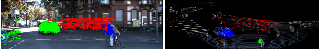
FIGURE 4.3 – Illustration of 2D-SSC and 3D-SSC for motion segmentation: the 2D-SSC approach (left) wrongly clusters the 2D feature trajectories of the road sign into the motion of the van. On the contrary, the 3D-SSC (right) is able to correctly cluster the 3D feature trajectories of the three moving objects, namely the background, the van and the cyclist.
