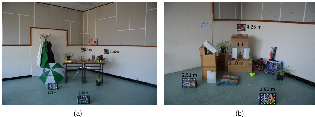
Figure 4.2: Scene A (a) and Scene B (b). The distances of different MCCs to the camera are shown. The resolution of the image is 6000×4000.
