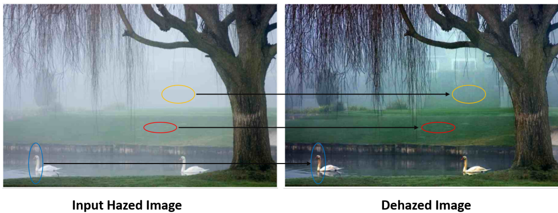
Figure 3.9: The color recovery of a hazy image treated by Tan's dehazing method. These images have been borrowed and modified from the Figure 10 of the paper of Tan [165].
