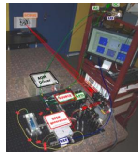
Fig. 2. Photograph of the setup where the path of light and of the signals delivered by the photodiodes (LO, DC, and AC) have been highlighted with color lines to provide a guide for the eyes.
