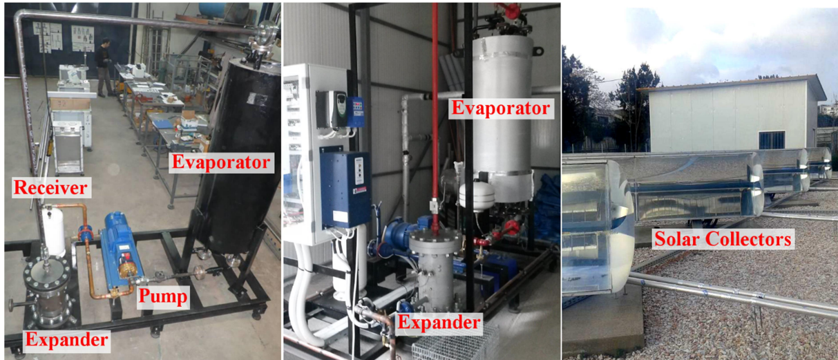
Figure III-3: CPV-Rankine installation pictures
