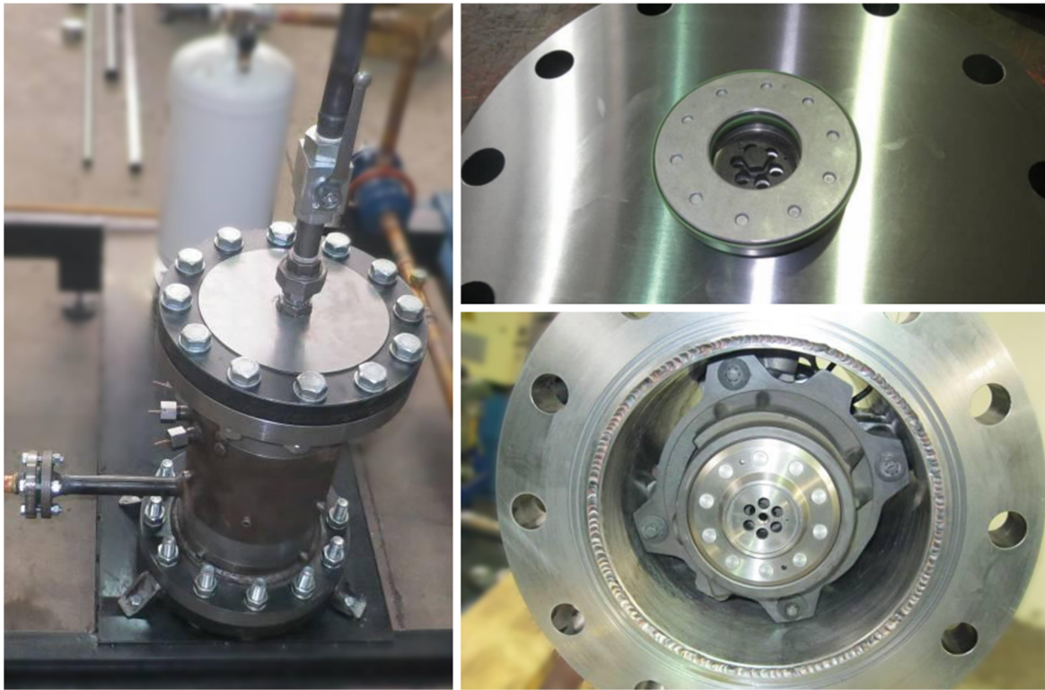
Figure VII-7: CPV-Rankine modified scroll expander
