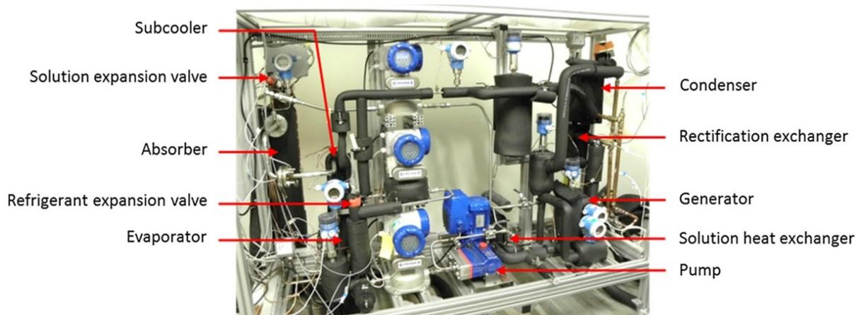
Figure III-8: Absorption chiller installation picture (Triché et al. 2017)
