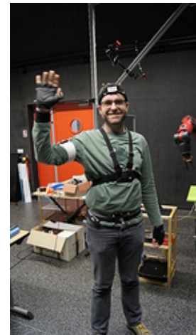
Figure 6.2: Optitrack suit for human tracking. The suit tracks the Cartesian location of the waist, trunk, head and both shoulder, elbows and wrists. To obtain the q vector of the model we perform an inverse kinematic.
