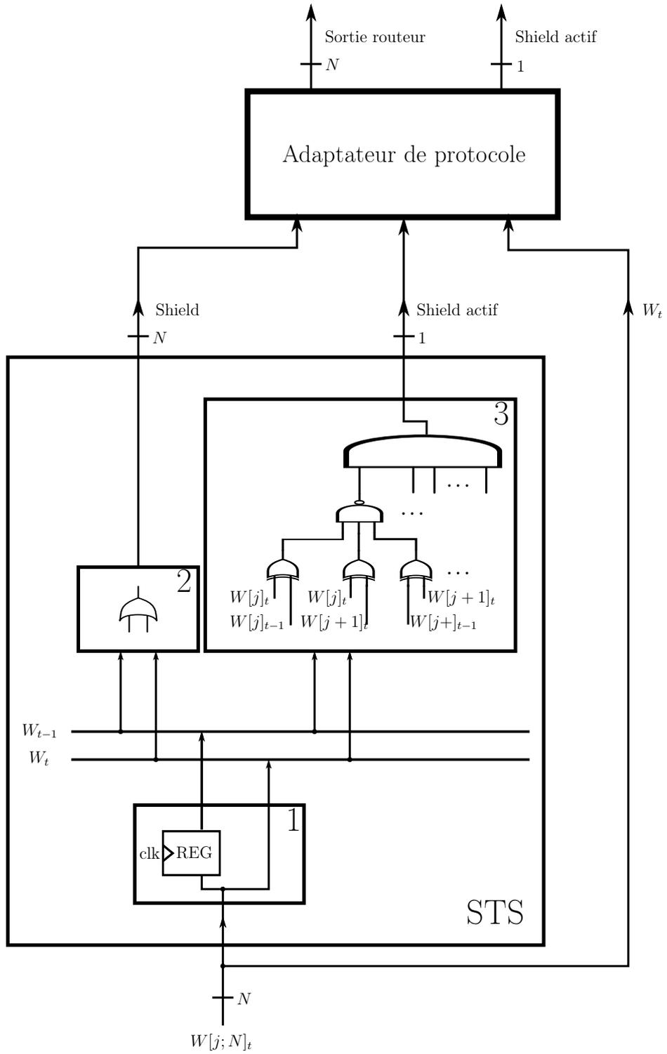
FIGURE 4.7 – Architecture du Smart Temporal Shielding (STS).
