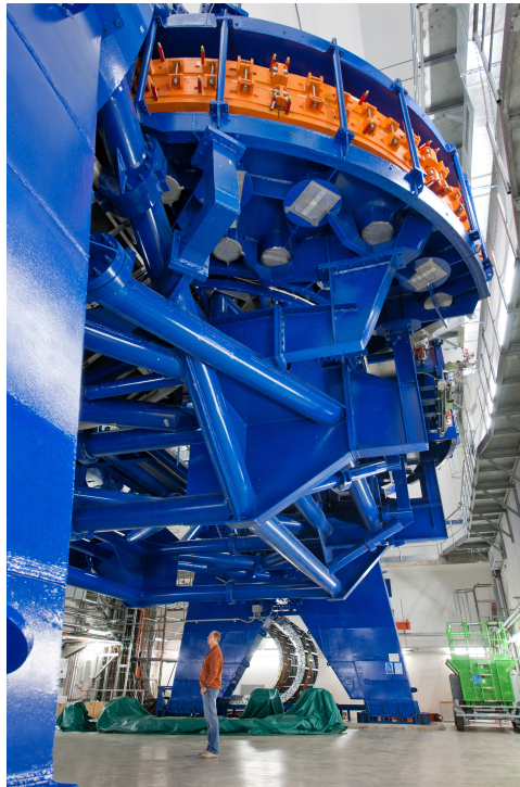
Figure 1.13: A photo of the gantry at the Heidelberg Ion-Beam Therapy Center (HIT), in the horizontal position. The support structures are painted blue and the bending magnets orange. Photo courtesy of Universitätsklinikum Heidelberg.
