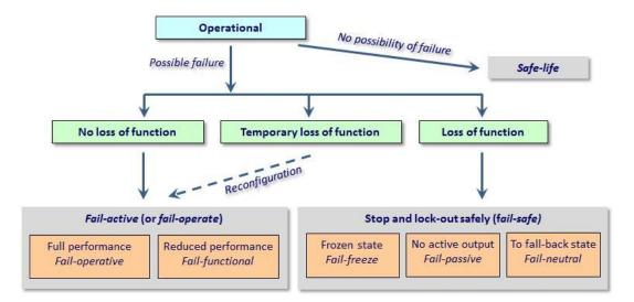
Figure 1.16 – System response to component failure [MAR16].
