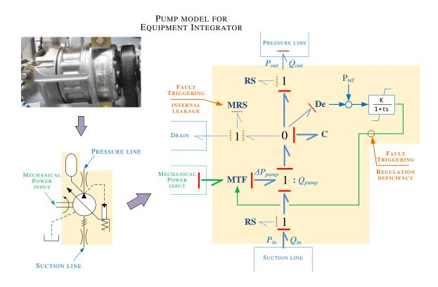
Figure 2.15 – Virtual Model: axial piston, variable displacement, pressure-regulated pump.
