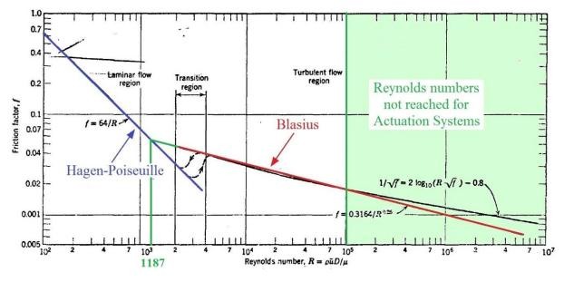
Figure 2.18 – Flow pattern in hydraulic lines from [MER67].
