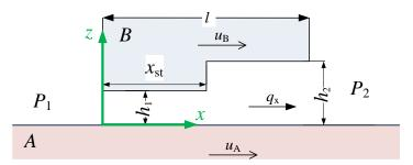
Figure 3.4 – Constant height gradient fluid film.
