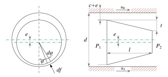
Figure 3.10 – Geometry and notations of a conical bearing from [VIE80].
