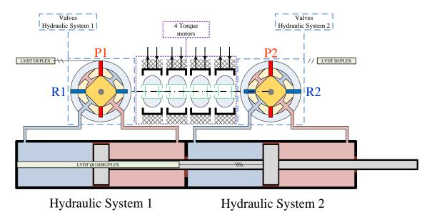
Figure 1.21 – NH90 Direct Drive Valve actuator.
