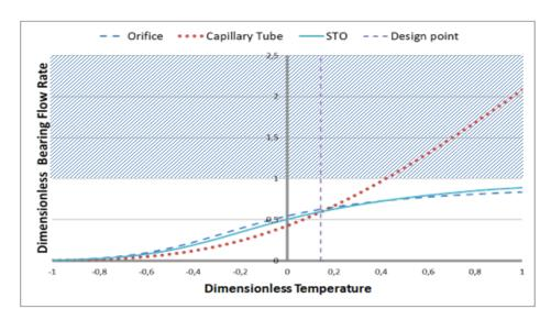
Figure 3.8 – Dimensionless bearing flow rate versus fluid temperature.
