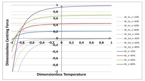
Figure 3.11 – Dimensionless centring force versus fluid temperature.
