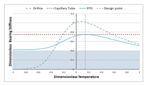
Figure 3.9 – Dimensionless bearing stiffness versus fluid temperature.
