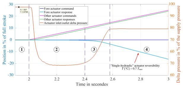
Figure 2.31 – Actuator response couplings.
