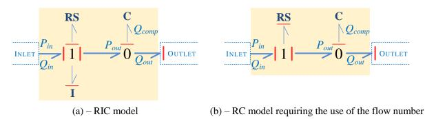
Figure 2.20 – Pipe virtual model used in our Actuation System modelling.
