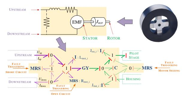
Figure 2.23 – Interface stage: electrical motor virtual model.
