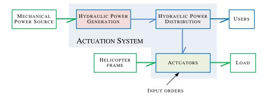
Figure 2.9 – Actuation System word Bond-graph.
