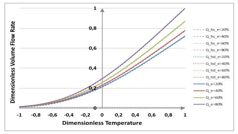
Figure 3.12 – Dimensionless volume flow rate versus fluid temperature.
