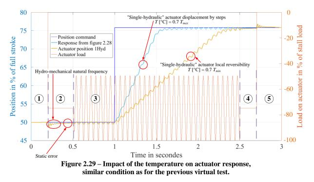
The single-hydraulic actuator response time is increased by a factor of nearly 2.5. The actuator is even driven backwards by the load. Indeed, in these moments, the actuator punctually and cyclically enters in reversibility (see *Note 2.14*). The back flow is observed in Figure 2.30<sup>22</sup> that shows both the volume flow rate and pressure drop at the valve orifice  $\sigma_{s\_ext}$  for the time period [1.5;1.65] (approximately) of zone ③.
