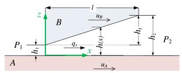
Figure 3.3 – Constant height gradient fluid film.
