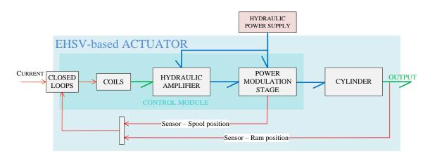
Figure 1.18 – EHSV based Actuator word Bond-graphs.
