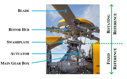
Figure 1.4 – Fixed and rotating references, main components near the rotor hub.
