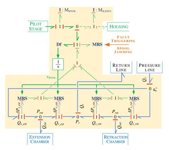
Figure 2.27 – Power modulation stage virtual model: hydro-mechanical valve.
