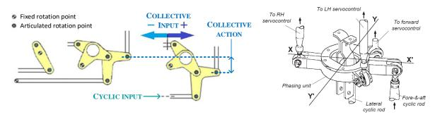
Figure 1.6 – Mixing unit on Alouette III from [SUD59].
