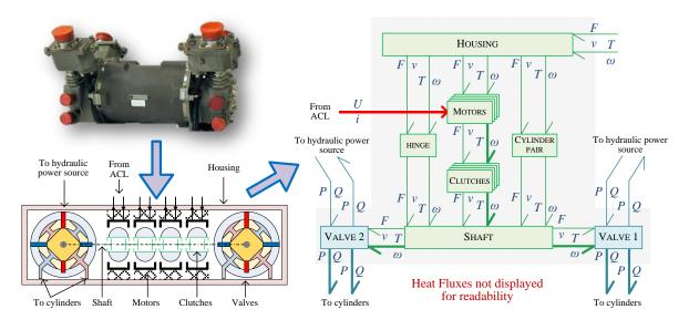
Figure 2.4 – Linking the model architecture to the system topology.
