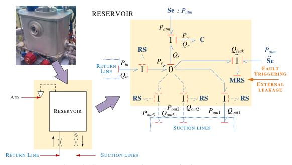
Figure 2.12 – Non-pressurized reservoir virtual model.
