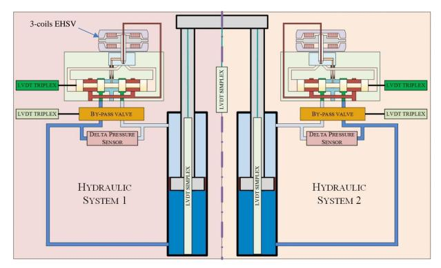
Figure 1.19 – EHSV based reference actuator.
