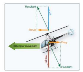
Figure 1.2 – Balanced forces in forward flight [FAA12].
