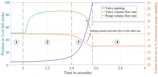
Figure 2.32 – Actuator response couplings: communicating flow rates.
