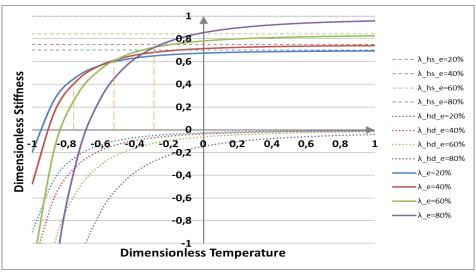
Figure 3.13 – Dimensionless stiffness versus fluid temperature.
