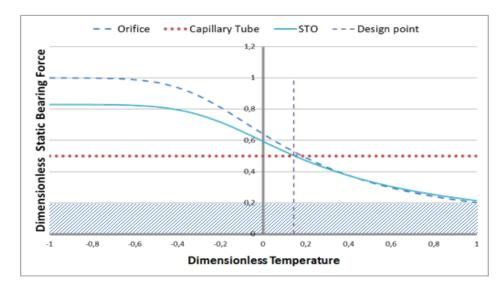
Figure 3.7 – Dimensionless static bearing force versus fluid temperature.
