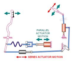
Figure 1.14 – SCAS actuation concept.
