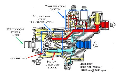
Figure 2.14 – Axial piston, variable displacement, pressure regulated pump from [MAR01].
