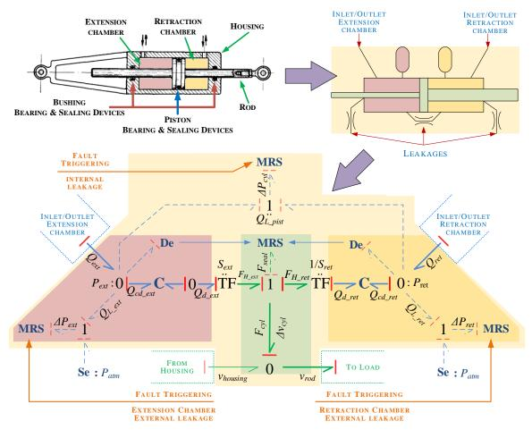
Figure 2.21 – Cylinder virtual model.
