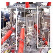
Figure 1.8 – Flight controls on Alouette III [SUD59].
