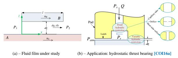
Figure 3.2 – Constant height fluid film.
