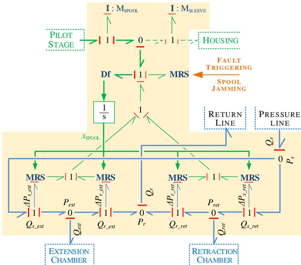
Figure 2.27 – Power modulation stage virtual model: hydro-mechanical valve.
