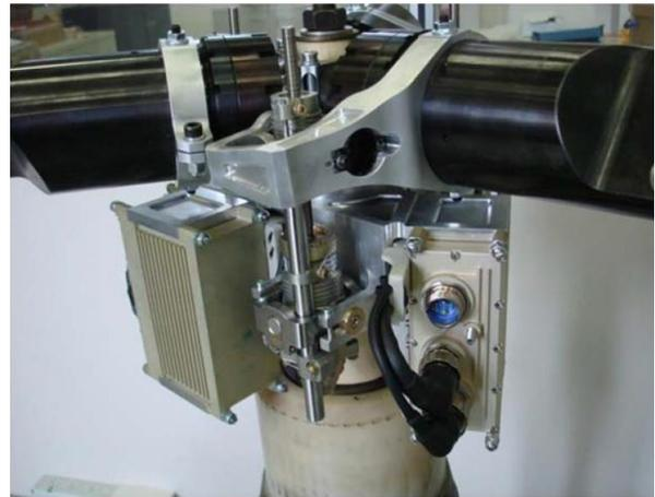
(a) IBC actuators on a UH-60 rotor head [HAB02] (b) IBC EMA on a Project Zero blade [GIA14]
