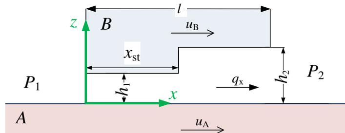
Figure 3.4 – Constant height gradient fluid film.
