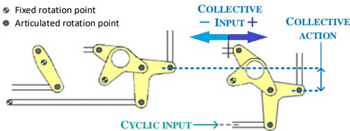
Figure 1.6 – Mixing unit on Alouette III from [SUD59].
