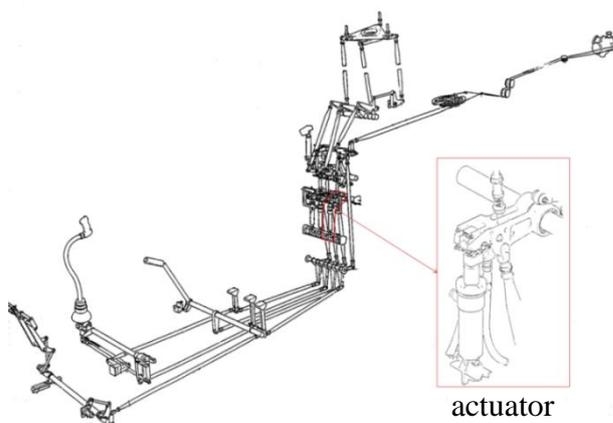
Figure 1.8 – Flight controls on Alouette III [SUD59].
