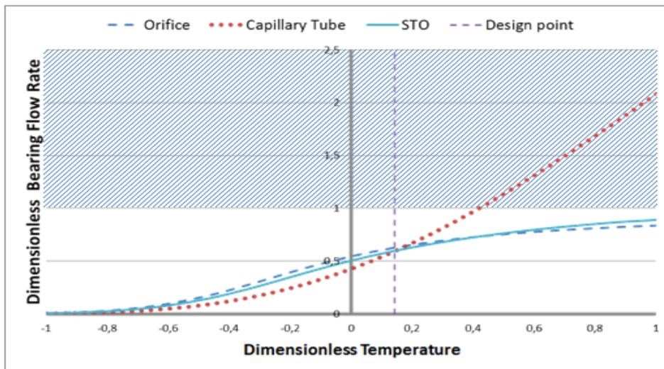
Figure 3.8 – Dimensionless bearing flow rate versus fluid temperature.
