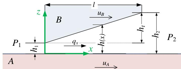
**Figure 3.3 – Constant height gradient fluid film.**
