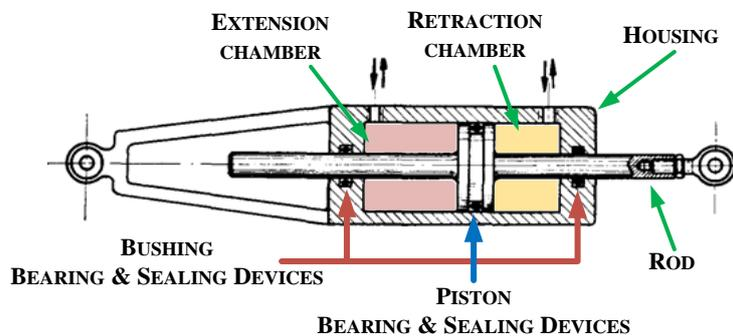
**Figure 1 – Dynamic bearing and sealing devices in a hydraulic cylinder, modified from [FAI06].**
