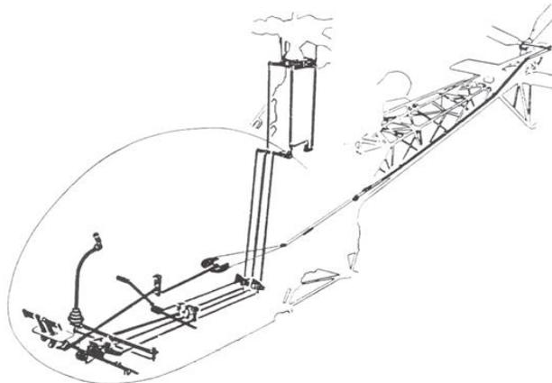
Figure 1.5 – Flight controls on Alouette II representation [SNC55].
