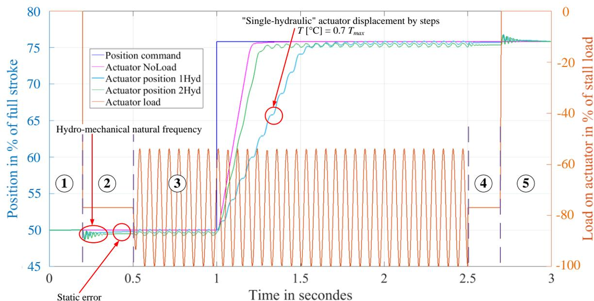
**Figure 2.28 – Impact of the load on actuator response, before and after the loss of one hydraulic system.**
