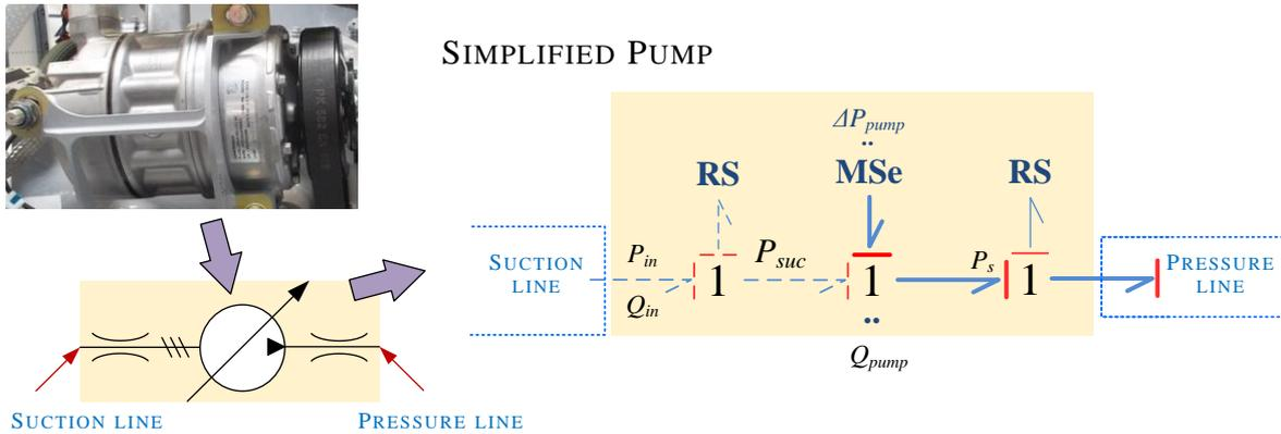
**Figure 2.13 – Variable displacement pump modelled as a combined effort source.**
