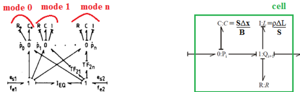
(a) – Obtained from modal analysis [LEB84] (b) – Segment to be repeated [PRS13]
