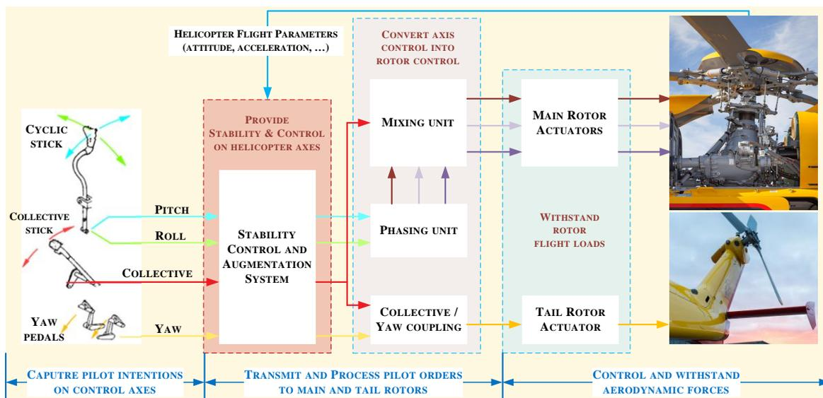
Figure 1.10 – Synthesis scheme of H/C flight control system with functional view.
