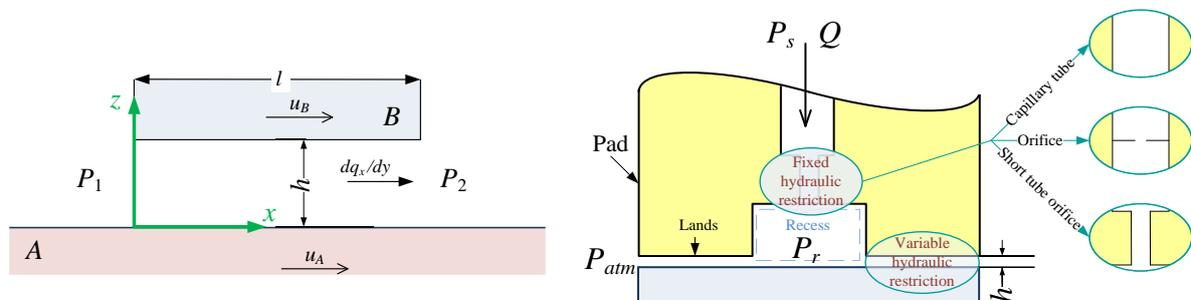
(a) – Fluid film under study      (b) – Application: hydrostatic thrust bearing [COI16a]
