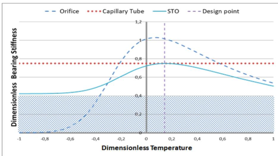
Figure 3.9 – Dimensionless bearing stiffness versus fluid temperature.
