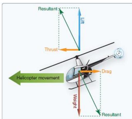
Figure 1.2 – Balanced forces in forward flight [FAA12].
