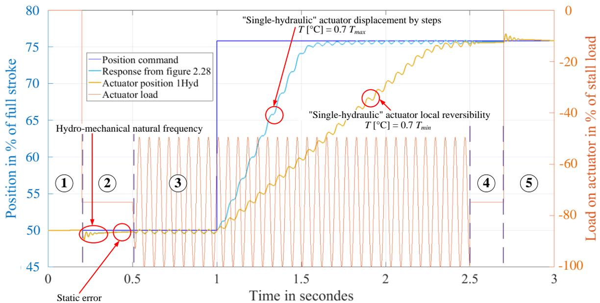
**Figure 2.29 – Impact of the temperature on actuator response, similar condition as for the previous virtual test.**
