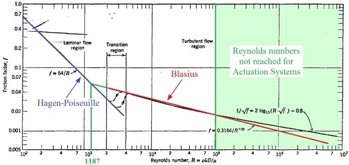
Figure 2.18 – Flow pattern in hydraulic lines from [MER67].
