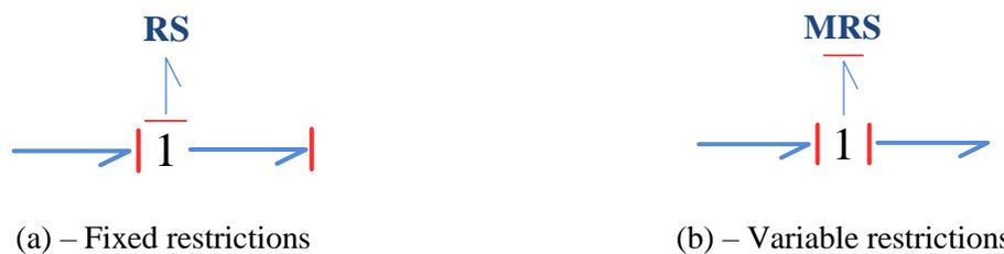
**Figure 2.16 – Preferred restriction causalities based on equations found in literature.**
