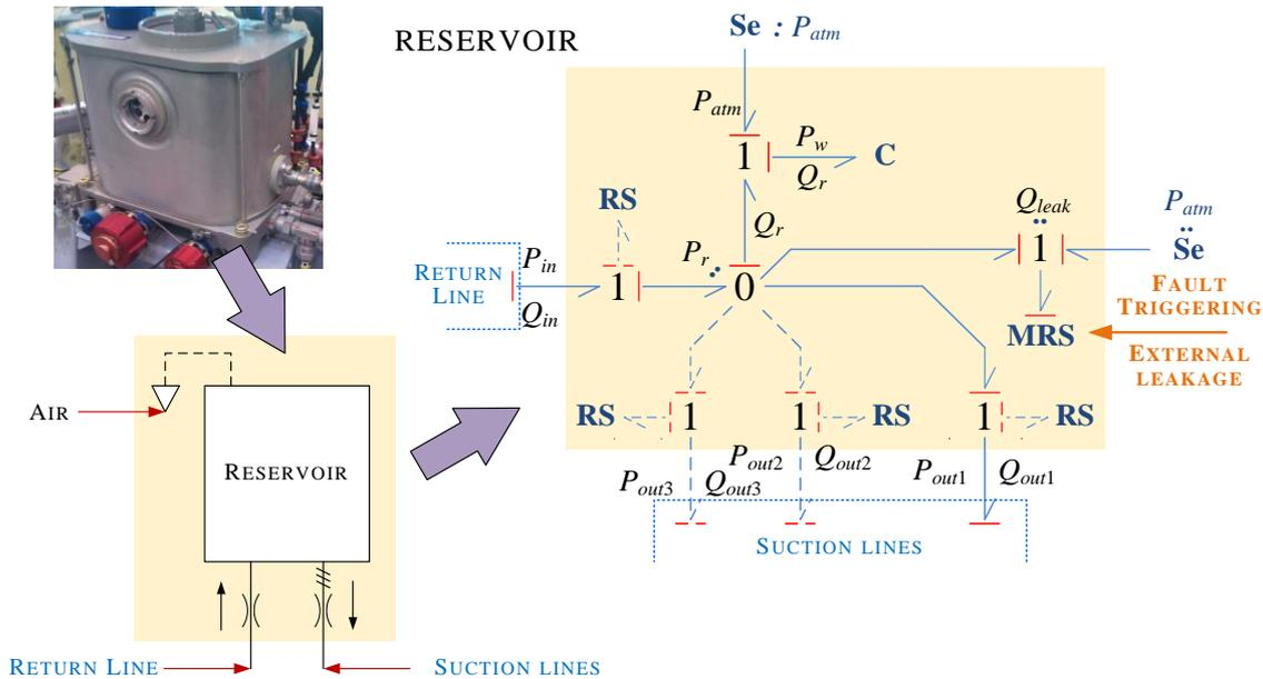
Figure 2.12 – Non-pressurized reservoir virtual model.
