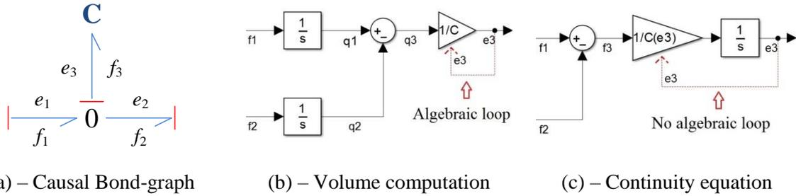
**Figure 2.8 – Bond-graph of a hydraulic capacitive effect and two possible implementations.**
