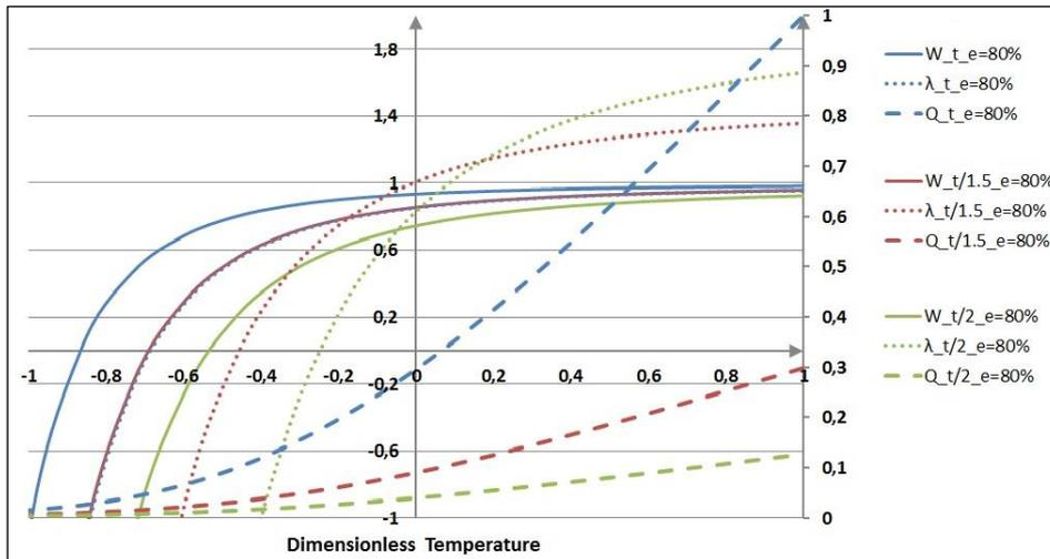
**Figure 3.15 – Dimensionless main criteria versus fluid temperature for different taper heights.**
