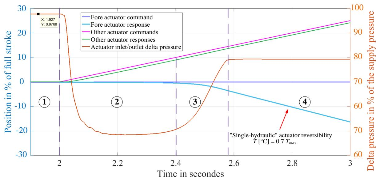
**Figure 2.31 – Actuator response couplings.**
