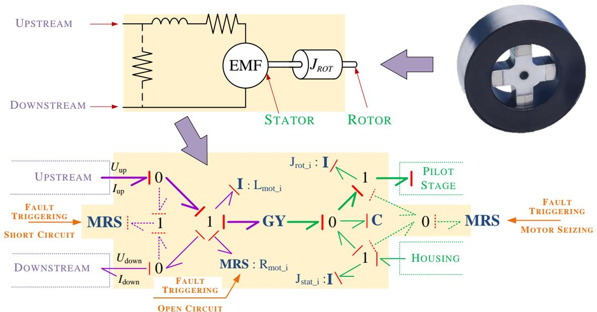
Figure 2.23 – Interface stage: electrical motor virtual model.
