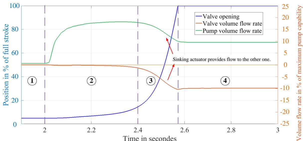
**Figure 2.32 – Actuator response couplings: communicating flow rates.**
