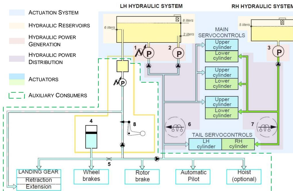
Figure 2.11 – H225 Hydraulic System with the main users identified from [EUR04].
