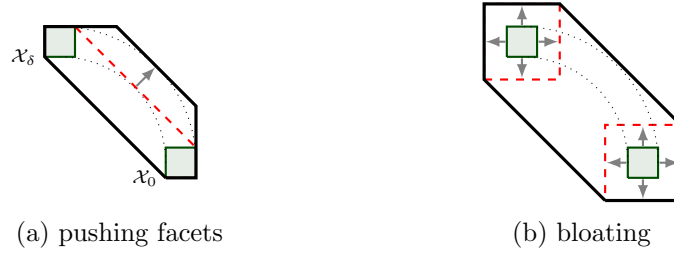
Figure 2.7: An approximation \Omega_0 that covers \mathcal{X}_t for t \in [0, \delta] can be obtained from the convex hull of \mathcal{X}_0 and \mathcal{X}_\delta and compensating for the curvature of trajectories
