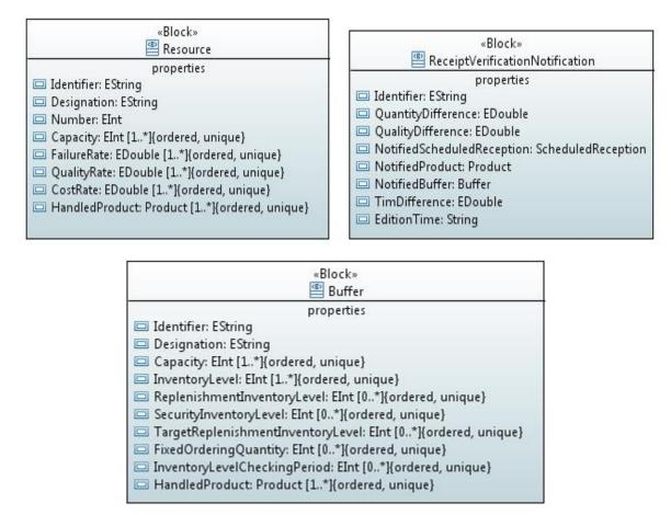
FIGURE A1.20: DETAILS OF THE USED IMPUTS AND OUTPUTS FOR THE VERIFY OPERATION
