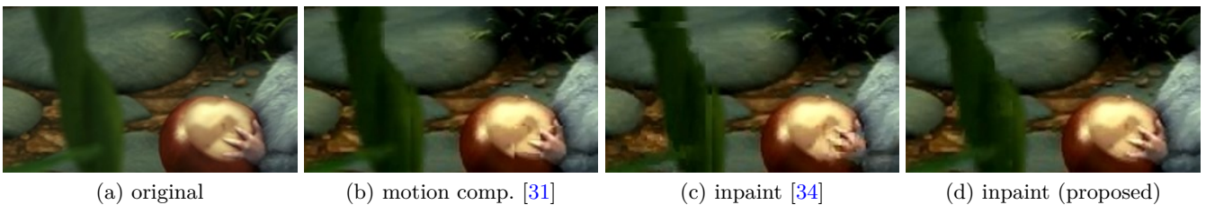
Figure 8.5 – Example 1: Comparison of different error concealment methods for 10% of lost of sequence 1 (pink rectangle).
