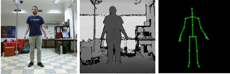
Figure 2.4 – Example of data provided by RGB-D sensors like Microsoft Kinect 2: 2D color image (left), depth map (middle) and 3D skeleton (right).
