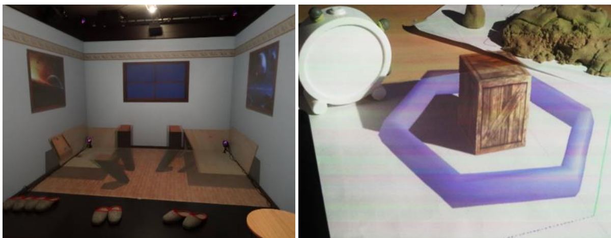
Figure 15: Spatial immersive augmentation: Square CAVE (left), dynamic perspective-corrected projection over an arbitrary environment (right, the box and the bluish hexagon are projected)
