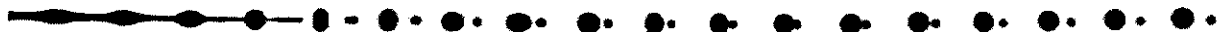
Figure 4-24 Illustration du phénomène de fusion réflexive. ( a = 220 \mu\text{m} , U_0 = 5,02 \text{ m/s} , f_{\text{tension}} = 898 \text{ Hz} , V = 1200 \text{ Volts} , d_{j-e} = 500 \mu\text{m} , \sigma = 58 \text{ mN/m} , \mu = 17 \text{ mPa s} , \rho = 1165 \text{ kg/m}^3 ).
