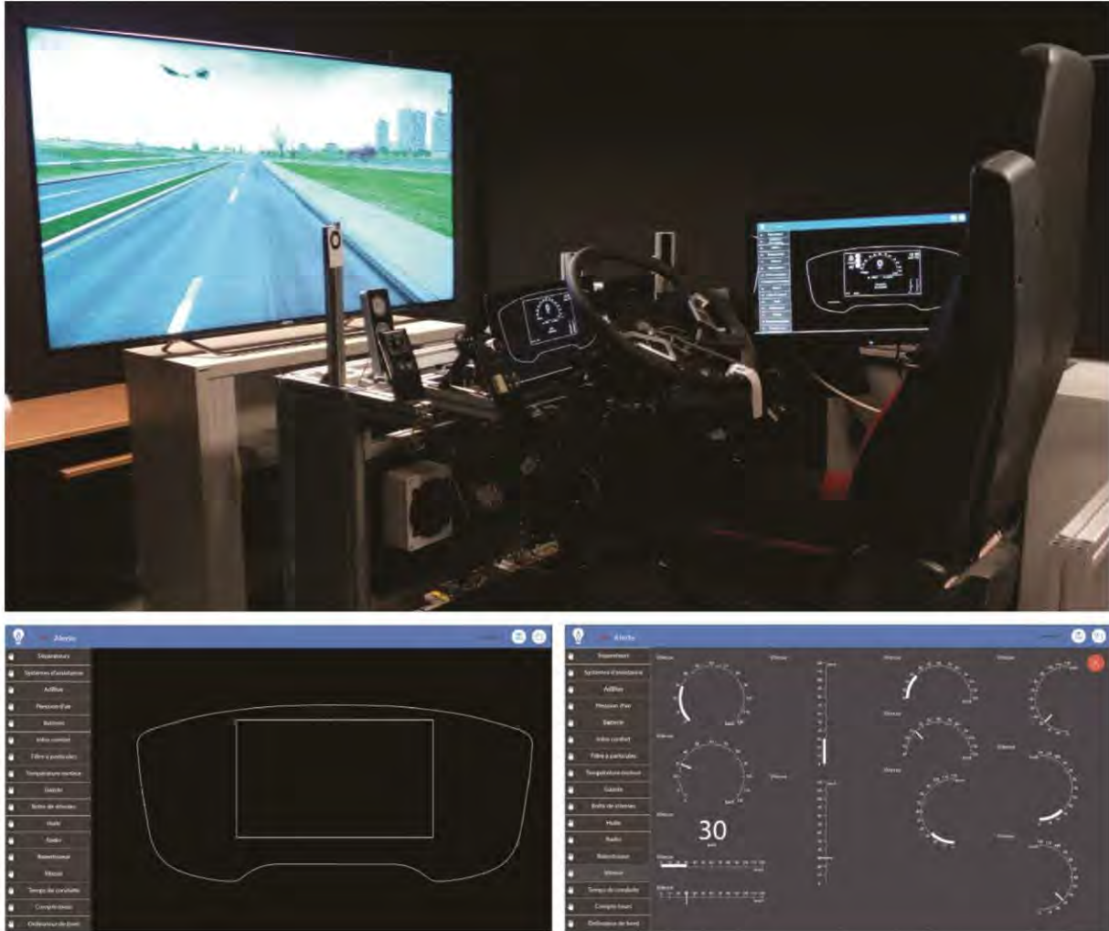
Figure 1. Equipment setup: on the driving simulator, users could design their interface on the touchscreen to the right. The dashboard was reported instantly and functionally behind the steering wheel. The software on the touchscreen is shown on the bottom images, the user chooses a function in the function panel on the left, and it opens a widget panel with all the representations available. Thus, he could choose a widget that was displayed on the stage. He could then change his size and location.
