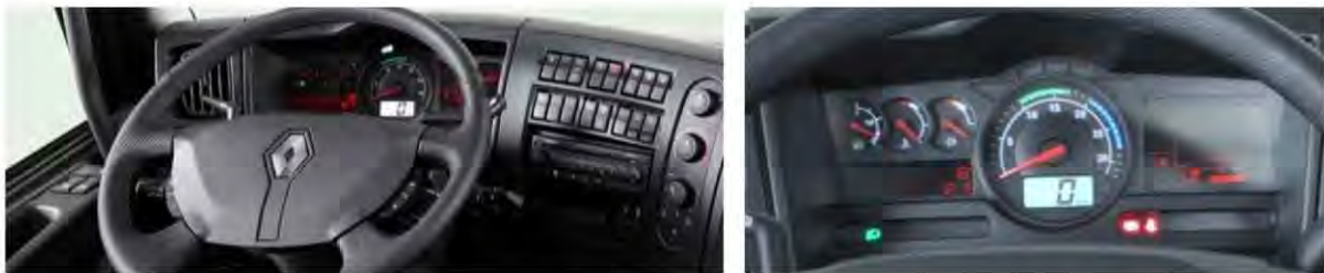
Figure 2. The instrument panel (common to the C, D wide, and D) and the instrument cluster (common to all MPV)
