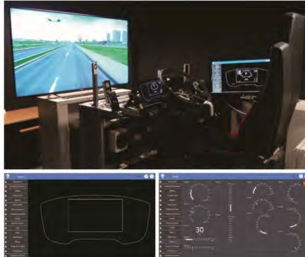
Figure 1. Equipment setup: on the driving simulator, users could design their interface on the touchscreen to the right. The dashboard was reported instantly and functionally behind the steering wheel. The software on the touchscreen is shown on the bottom images, the user chooses a function in the function panel on the left, and it opens a widget panel with all the representations available. Thus, he could choose a widget that was displayed on the stage. He could then change his size and location.
