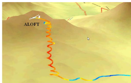
Figure 2.12: Spiral-shaped flight trajectory during thermal centering flight, [3]
