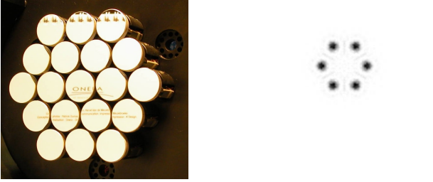
Fig. 11. Left: the active segmented mirror with 19 sub-apertures. Right: Simulation of the parking position in the focal plane with the 6 sub-apertures used (first corona).
