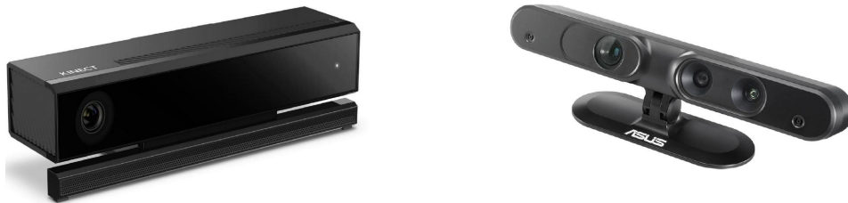
Figure 2.6 – Example of RGB-D sensors. Left: Microsoft Kinect 2 [61], right: Asus Xtion PRO LIVE [3].
