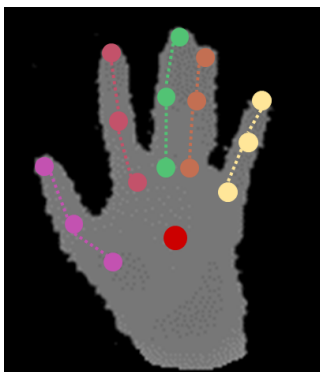
Figure 5.2 – A hand depth image and its K 3D joints. Here, K equal to 16: 3 joints by fingers and one for the palm.
