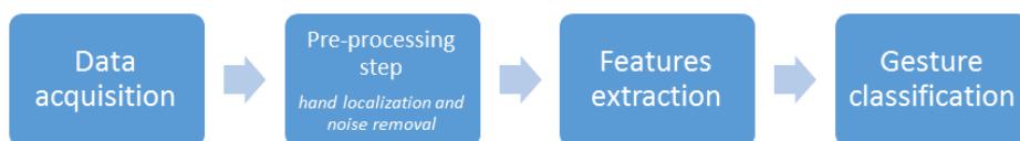
Figure 2.3 – The pipeline of vision-based traditional hand gesture recognition systems. First, visual data are captured. Second, an optional pre-processing step is often conducted in order to extract the region of interest of the hand from the background. Third, features are computed to extract relevant hand gesture information. Finally, a classification step outputs a label.
