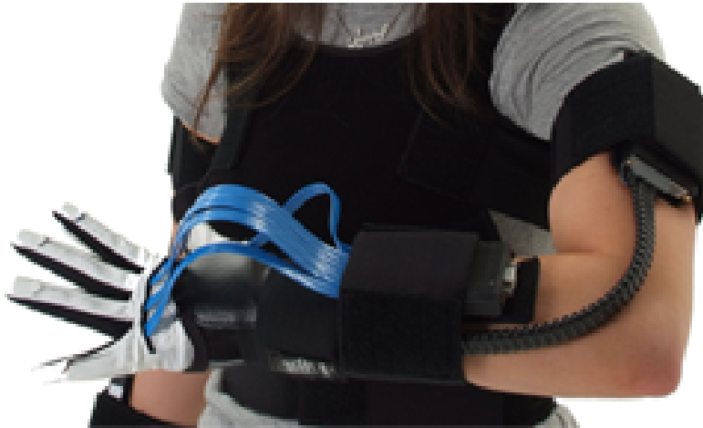
Figure 2.10 – The ShapeHand [131] glove motion capture systems.
