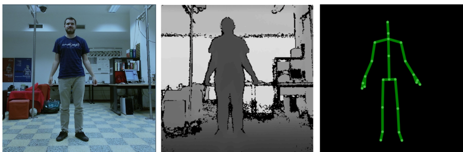
Figure 2.7 – Example of data provided by RGB-D sensors as Microsoft Kinect 2 [61] : 2D color image (left), depth map (middle) and body 3D skeleton (right).
