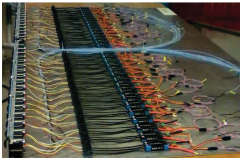
Fig. 4. The 32 motors actuating the AEA prototype
