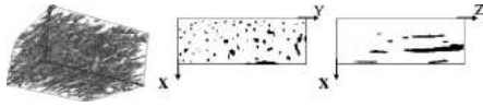
FIG. 1. Three-dimensional porous network (pores are in grey) in a parallel-pipedic block extracted from the \mu CT reconstructed bone structure. On the right-hand side are shown a transverse and longitudinal cross section through the three-dimensional porous network. The preferential orientation of the pores is along the bone axis.
