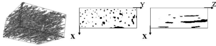
FIG. 1. Three-dimensional porous network (pores are in grey) in a parallel-pipedic block extracted from the \mu CT reconstructed bone structure. On the right-hand side are shown a transverse and longitudinal cross section through the three-dimensional porous network. The preferential orientation of the pores is along the bone axis.
