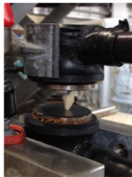
FIGURE 1.9 – Resonant ultrasound spectroscopy set-up.
