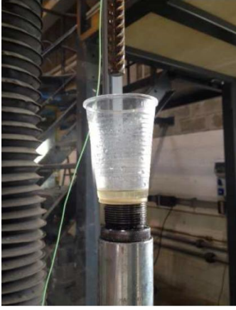
Figure 3-29: Water flow along rebar during heating at 100 and 140°C (Toumi Ajimi et al., 2015)
