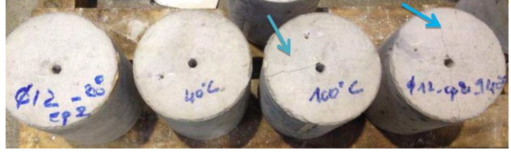
Figure 3-30: Cracks observed for concrete at 100 and 140°C (Toumi Ajimi et al., 2015)
