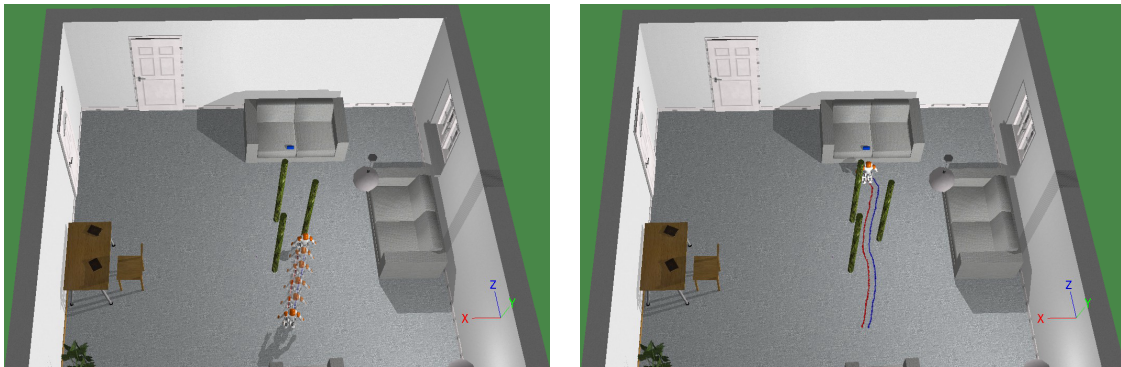
Figure 6.15 – Non-reactive vs. reactive approach. On the left Reactive Motion is deactivated. Some frames capturing the evolution of the robot are superimposed. The robot ended up blocked by the obstacle. On the right, with the activation of Reactive Motion the agent is able to accomplish the task.
