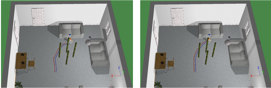
Figure 6.27 – CS-II vs CS-III implementation. On the left, the result for CS-II where a single walk mode was available. On the right, the results for the current implementation, so a dual walk scheme based on visual encoding arbitration was available.
