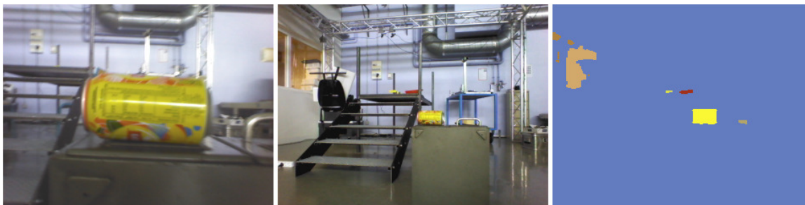
Figure 4.24 – Multi-color saliency. On the left, a closeup view of a tracked object, which corresponds to a colored can with different tonalities of yellow and orange. In the center, the scene registered on-board from distance. On the right, several regions are salient in segmentation, due to the color diversity of the object model. Hence, a problem to be solved is selecting the correct salient region on the segmented image.
