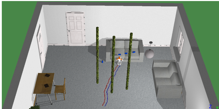
Figure 6.28 – Evaluation of the condition of multiple objects and obstacles. Despite the presence of other cans on the sofa, the robot was able to approach the desired one by relying on the embodied filtering process (described in Sec. 5.4).
