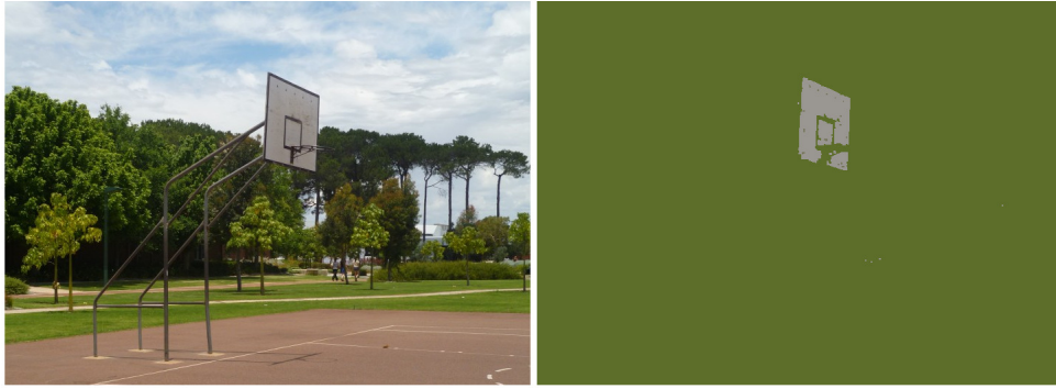
Figure 3.15 – Segmentation of a natural scene. On the left the original image. On the right the segmentation of the backboard.
