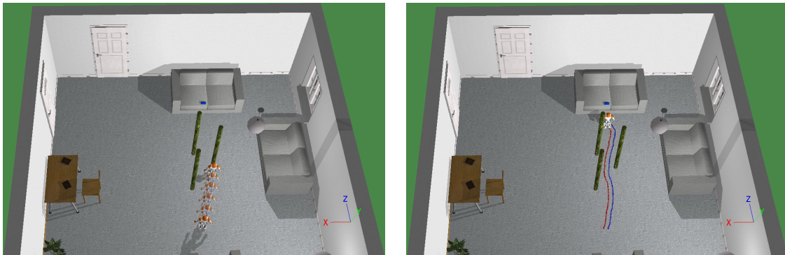
Figure 6.15 – Non-reactive vs. reactive approach. On the left Reactive Motion is deactivated. Some frames capturing the evolution of the robot are superimposed. The robot ended up blocked by the obstacle. On the right, with the activation of the Reactive Motion the agent is able to accomplish the task.
