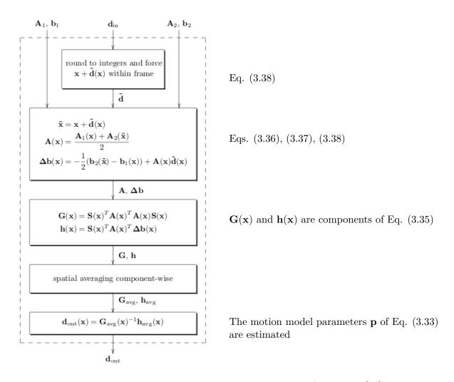
Figure 3.18 – Algorithm for displacement estimation (Farnebäck [69]).
