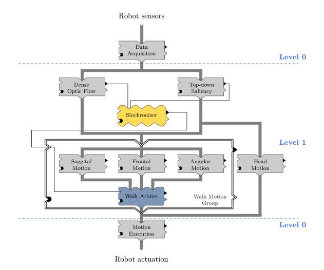
Figure 6.5 – Two-level hierarchy model. The level 0 corresponds to the real sensory and motor data. Virtual sensors and behavior primitives are defined in the level 1.
