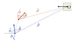
**Figure 4.3** – Top view of the localization prediction. The parameter  $\iota$  is not shown since it is assumed do be constant. The heading direction of the object is shown in black. The motion direction of the agent is shown in blue. The prediction  ${}^B\tilde{\zeta}$  from Eq. (4.17) is shown in orange.
