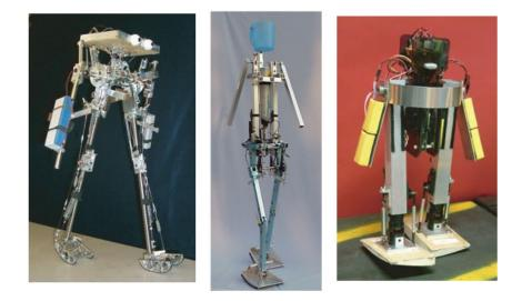
**Figure 2.8** – Passive dynamics research. Three level-ground powered walking robots based on the ramp-walking designs (Collins et al. [49]). On the left the Cornell biped, in the center the Delft biped, on the right the MIT learning biped.
