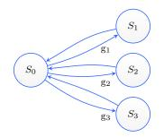
**Figure 6.20** – State automate for discrete events arbitration between the motion profiles described in Tab. 6.5. The transition events are denoted by  $g_i$ , which are described in Tab. 6.6.
