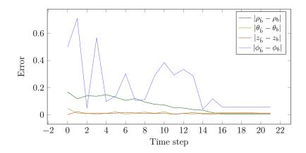
**Figure 4.10** – Evolution of the localization error between the estimations  $\hat{b}$  and the measurements b.
