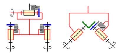
**Figure 2.6** – Nao's pelvis design. On the left the classical set of three rotary joints, one horizontal axis at the waist and two vertical axis for the legs. On the right the coupled inclined axis rotary joints (at  $45^{\circ}$  towards the body) for the Nao pelvis (Gouaillier et al. [75]).
