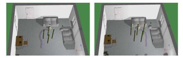
Figure 6.17 – Evaluation of motion consistency. During the approach the agent losses the view contact with the object of interest, so it has to rely on the temporarily persisted locations.
