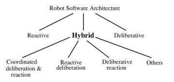
**Figure 2.13** – Architectures for mobile robot control. Classification of mobile robot control architectures in Pirjanian [145].
