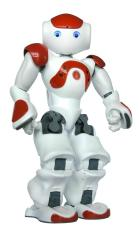
Figure 2.5 – The robot Nao by Aldebaran Robotics (Gouaillier et al. [75])
