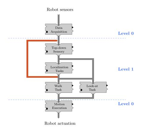
**Figure 6.6** – Equivalent iB2C model for the behavior scheme describes in Sec. 5.3. The Sensory and Localization tasks were grouped in single nodes for simplicity. The orange arrow corresponds to the feedback sent for predicting the evolution of the embodied features detailed
