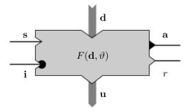
Figure 6.1 – Basic iB2C behavior module (Proetzsch et al. [152]).
