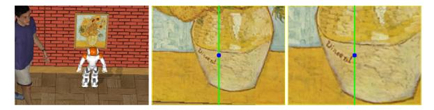
Figure 6.12 – On-board view of the sparse flow evaluation. In case the robot is critically proximal to the object, the centroid flow is no longer informative for the Saggital Motion behavior.
