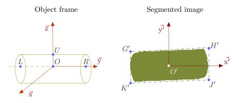
**Figure 4.6** – Cylindrical object model. On the left the 3D model of the object, the placement of frame O, and the definition of four points of interest. On the right the segmented blob and the definition of image features from the oriented bounding box.
