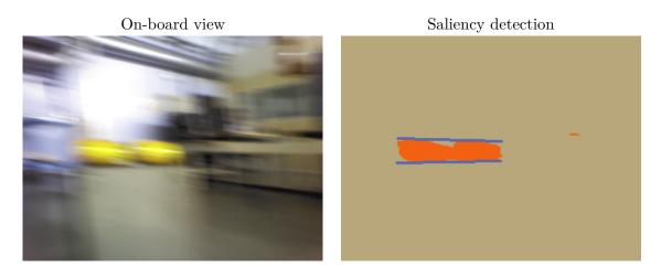
Figure 5.15 – On-board view of the experimental modality of continuous motion. Saliency degradation due to the view angle to the cans and the motion blur produced.
