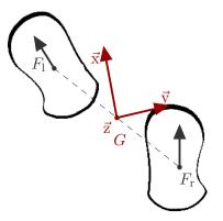
**Figure 4.13** – Definition of the ground frame. The frame G is placed at center of the projection of the feet in the ground. The z-axis is taken perpendicular to the ground, the x-axis is the mean direction obtained from the projection of the orientation  $F_1$  of the left foot and  $F_r$  of the right foot on the motion plane.
