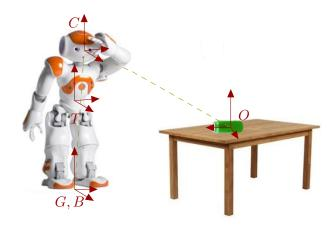
**Figure 4.1** – Definition of the reference frames to solve the localization task. G corresponds to the walk primitive frame, B is the movable reference frame for the Walk task (in the figure it coincides with G, though in Sec. 4.6.3 different locations for B are studied), C is the camera frame, T is the torso frame, and O is the object frame.
