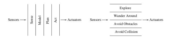
**Figure 2.16** – Comparison between deliberative and reactive models (Pirjanian [145]). On the left, the deliberative pipeline between the sensory input and the actuation on the environment. On the right, the concurrent execution of specialized programs so behavior emerges out of their conjoint actions.
