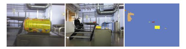
Figure 4.24 – Multi-color saliency. On the left a closeup of the object of interest: a colored can with different tonalities of yellow and orange. In the center the scene registered on-board. On the right different regions were salient due to the diversity of the color model.
