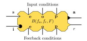
**Figure 6.3** – Structure of the CBS module (Armbrust et al. [10]). Three different types of ports (Enabling, Ordering, and Permanent) for input conditions (top) and feedback conditions (below). As a CBS is a behaviour, it also features the standard behaviour ports.
