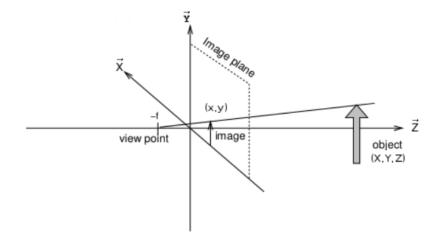
Figure 3.7 – Central perspective geometry (Corke [53]).
