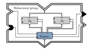
Figure 6.2 – Illustration of a group behavior interface (Proetzsch et al. [152]). Internally the outputs of two behaviors are combined in the fusion behavior represented in blue.
