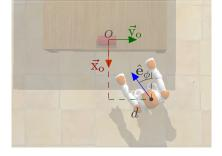
**Figure 5.1** – HMW non-holonoic angular motion. The lateral distance with respect to the object is denoted by d. O is the object frame origin. The direction of the saggital plane of the robot is shown in blue.
