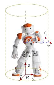
**Figure 4.5** – Representation of the ego-cylinder localization. In the image, *B* corresponds to the base frame, and  $\zeta$  represents the localization of an object in the environment. The heading direction  $\phi$  is represented emerging from the cylinder's surface.
