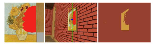
Figure 6.11 – On-board view of the bilateral symmetry condition. On the left the painting's texture is changed to generate a perceived asymmetric blob. In the center the features are marked. The centroid of the bounding box is plotted in blue and the vertical axis is green. On the right the salient blob. The on-board view corresponds approximately to the situation of "Frame a" in Fig. 6.10.
