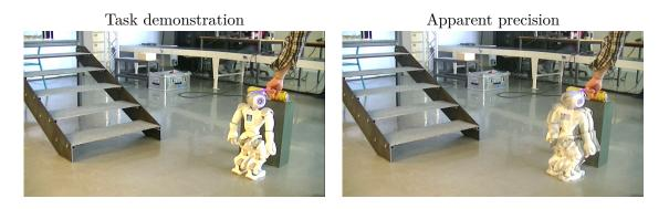
Figure 5.14 – On the left the demonstration of the desired pose in relation to the can. On the right the final position of some trials are superimposed.
