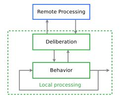
Figure 5.5 – Hybrid task architecture. The deliberative process evaluates the consistency of the autonomous local execution of the behavior. Once inconsistency is detected, remote processes are queried for support.
