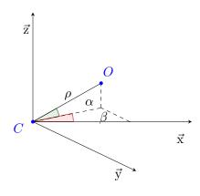
**Figure 4.4** – Illustration of the Look-at task. The center of the object is denoted by O. After the head correction, the x-axis of the camera frame C will be aligned with the direction  $\overline{CO}$ .
