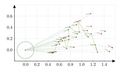
**Figure 4.9** – Egocentric visualization of the localization as perceived in B. The circumference represents the ego-cylinder. In red the real values, in green the estimations. Distances are expressed in m.
