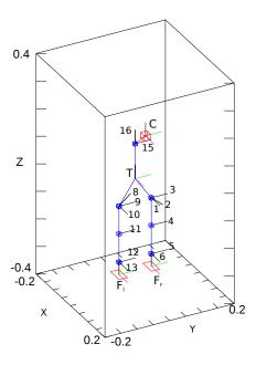
**Figure 4.12** – Geometrical model of the robot Nao. Distances are expressed in m. The orientation of the z-axis are projected in black along the structure. For the base frame T and the effector frames C,  $F_{\rm l}$ , and  $F_{\rm r}$ , the x- and y-axis are also plotted in magenta and green respectively. The active joints are numerated and represented by blue boxes. The effectors are represented in red.
