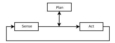
Figure 2.17 – The hybrid model principle (Morphy [131]). The sequence implies that, the robot first plans how to accomplish a mission or a task based on a global world model, and then activates a set of behaviors to fulfill the plan that is executed until it is completed.
