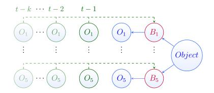
**Figure 5.8** – Dynamic policies for the Bayesian network. In green the past observations  $O_{i(t-1, \dots, k)}$ . These nodes don't belong to the actual network, the gradual fading of the color illustrates a decaying contribution (taking  $\gamma < 1$ ) according to recency (see Eq. (5.10)). In red the dynamically updated nodes  $B_i$ .
