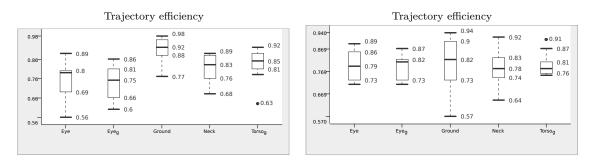
Figure 4.20 – Comparison on  $T_{\text{eff}}$  for experiments 1 (left) and 3 (right). In the experiment 3 the angular motion of the agent was obtained by the regulation of the yaw position of the neck, and noise was added to the proprioceptive measurements.
