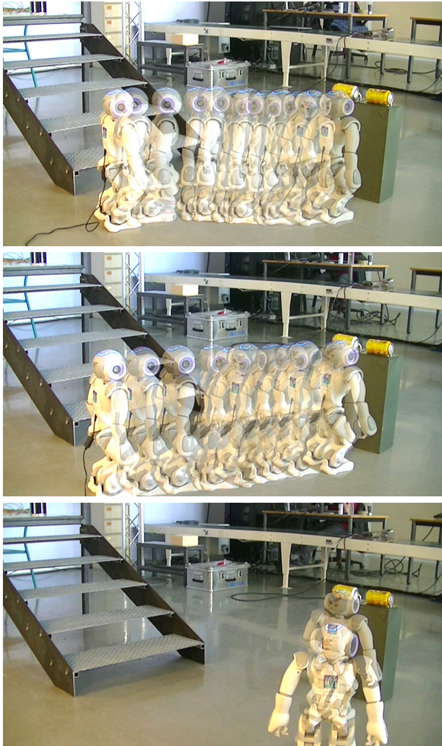
Figure 5.16 – Experimental evaluation with object redundancy. The sequences for three trials are shown. The robot was required to approach the can on the right.
