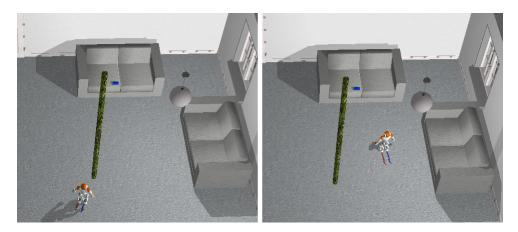
Figure 6.24 – Example of kinesthetic demonstrations for learning the scene encoding transitions. The robot walks towards the object. On the left a column is blocking the path, whereas on the right there is a free access to the object.
