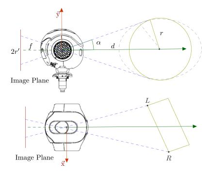
**Figure 4.7** – Estimation of the object's depth. On the top, the model assumes a view perspective  ${}^{C}\mathbf{o}_{\phi} = \pi$ . Bellow, the  $\vec{x}\vec{z}$  visualization of the scenario, where the circumference corresponds to an ellipse and the distance from the projective ray and the center of frame O is larger than r.
