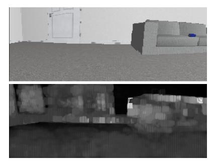
Figure 6.26 – Panoramic flow detection. On the top, the view of the scene at a range of  $\pi$  rad in the frontal ego-space. On the bottom, the normalized magnitude of the flow. Clearer regions should be phisically closer to the sensor than darker regions. As seen, noise from texture mapping in the simulated images affected the computation of the optic flow (e.g. the top-left corner of the sofa is perceived closer than the frontal part).
