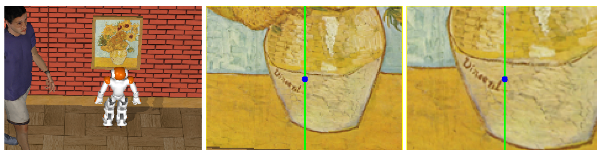
Figure 6.12 – On-board view of the sparse flow evaluation. In case the robot is critically proximal to the object, the centroid flow is no longer informative for the Saggital Motion behavior.
