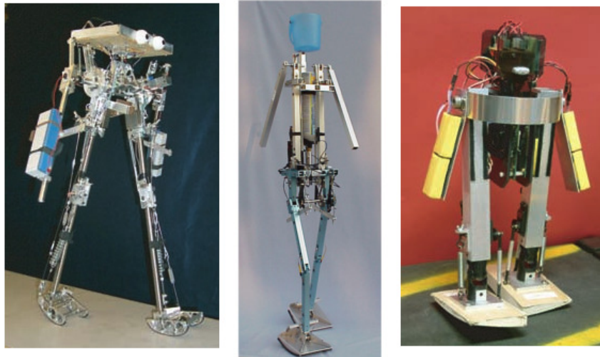
Figure 2.8 – Passive dynamics research. Three level-ground powered walking robots based on the ramp-walking designs (Collins et al. [49]). On the left the Cornell biped, in the center the Delft biped, on the right the MIT learning biped.
