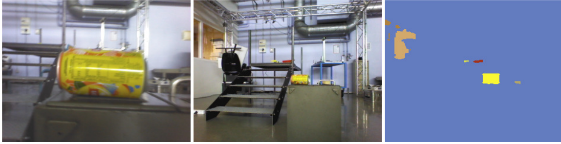
Figure 4.24 – Multi-color saliency. On the left a closeup of the object of interest: a colored can with different tonalities of yellow and orange. In the center the scene registered on-board. On the right different regions were salient due to the diversity of the color model.
