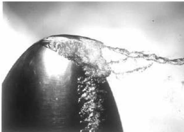
Figure I. 12 : Cavitation de tourbillon [Arndt, 2006]
