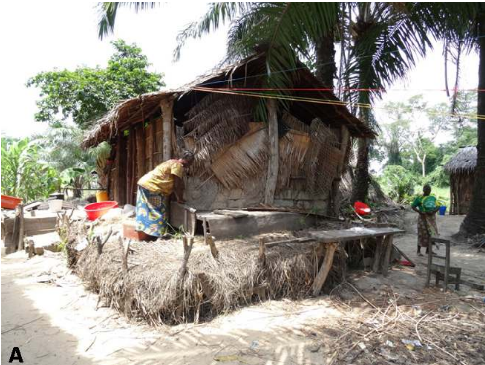
A: In the flood plain, people build earth mounds to protect their dwellings from seasonal flooding © M. COMPTOUR 2015
