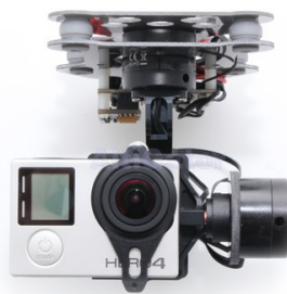
(a) Nacelle DYS 3-axes. Source : www.altigator.com
