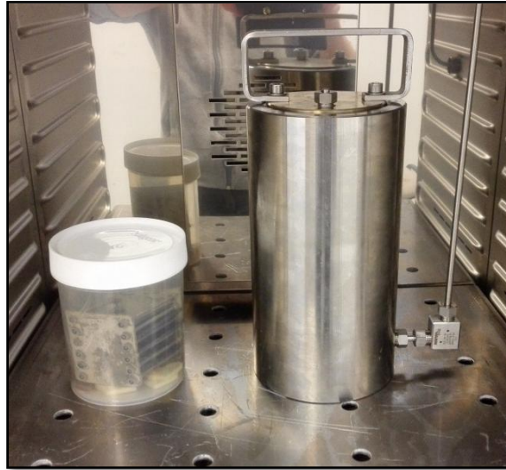
Figure 20 : (Left) 1 bar reference (Right) Test performed at 500 bar inside 40°C oven
