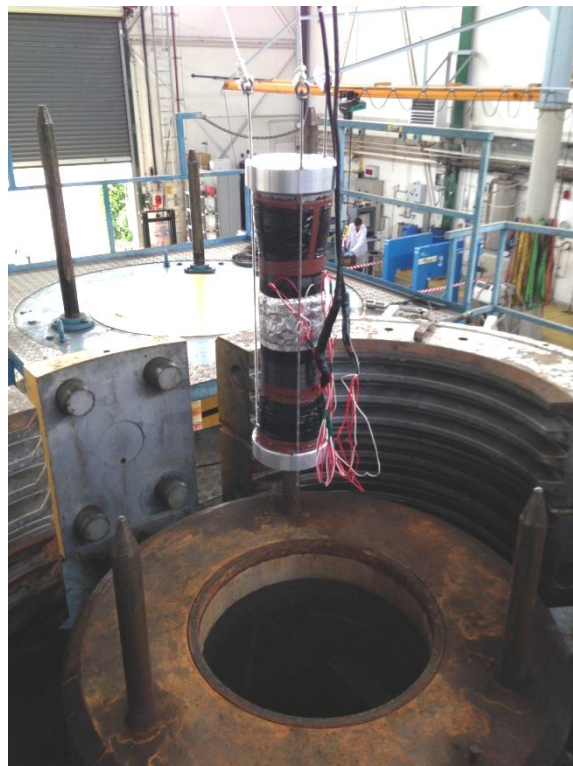
Figure 118 : Instrumented cylinder being lowered into the pressure vessel
