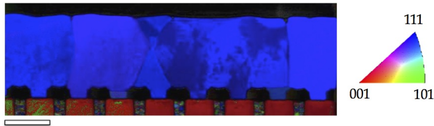
Figure 80: ACOM mapping of the cross-section of an as-is module, showing a strong \langle 111 \rangle texture of the Al grains along the deposition direction. The standard stereographic triangle gives the color codes of the grain orientations, taken here along the vertical growth direction. Scale bar 2.5 \mu\text{m} .
