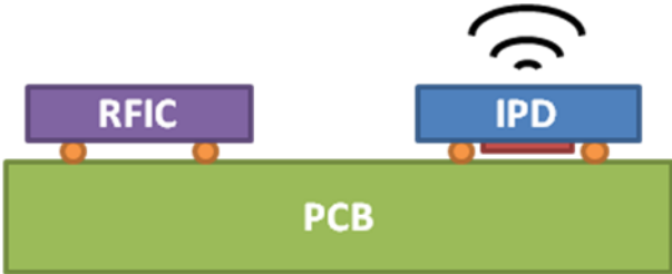
Fig. 46 Direct integration of the antenna and the RFIC into the PCB using the IPD process.
