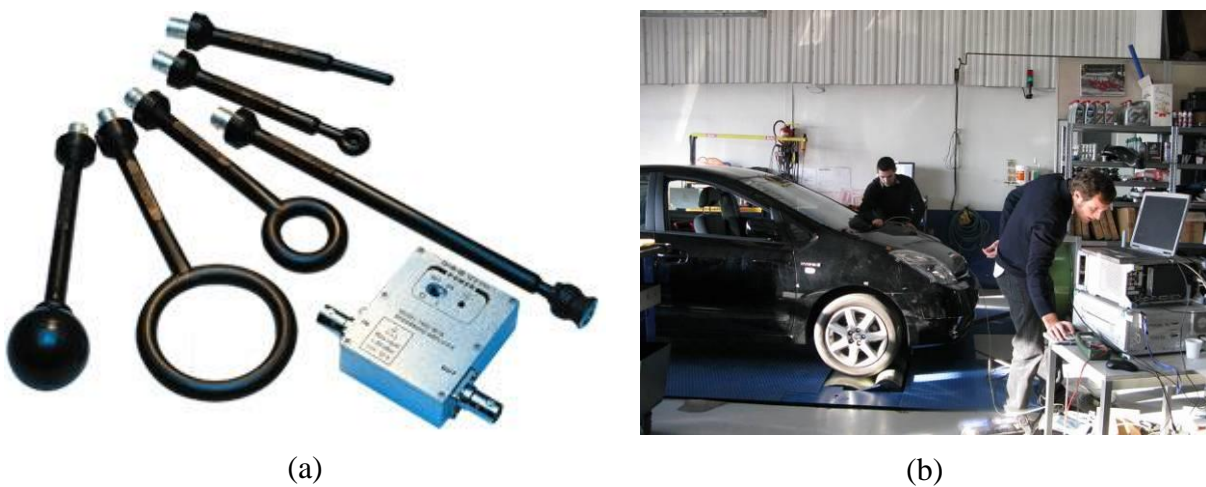
Fig. 14 (a) Probe field, (b) Probe measurements method
