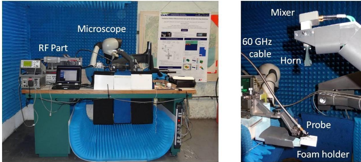
Fig. 90 Pictures of the measurement setup (Global view and closer view).
