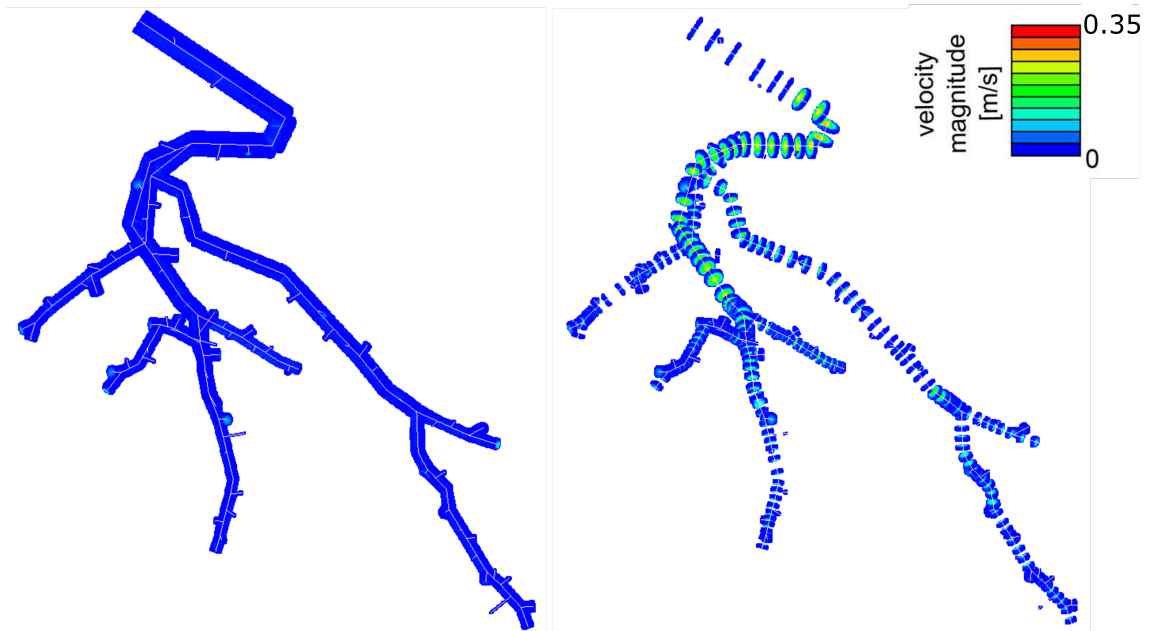
Figure 5.4: LBM blood simulation in the patient-specific arterial tree of Patient 2. Vessels with diameter > 2 mm represent the simulation domain. On the left, the vessels borders, where velocity is zero due to no-slip conditions, are visible. On the right image, regular slices of the vessels illustrate velocity at the interior of the vessels
